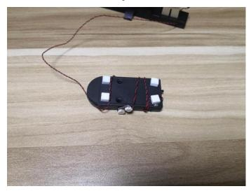
Stick the battery pack to the back of the name plate.
