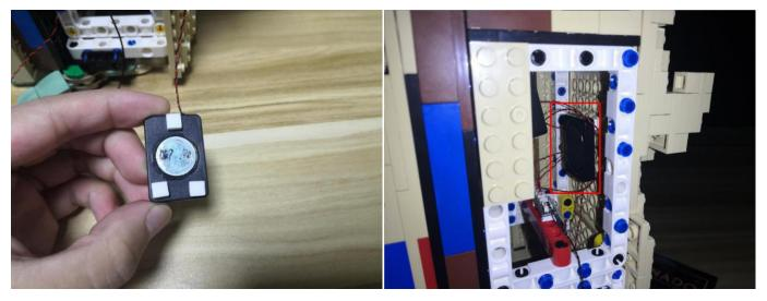
Stick an adhesive square to the receiver, stick the receiver to the following place.
