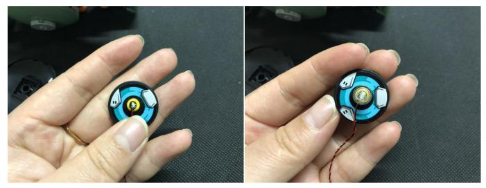
Thread the cable through the hole at the center of the black round piece.
