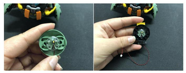
Reconnect the roof, connect the cable to the expansion board
