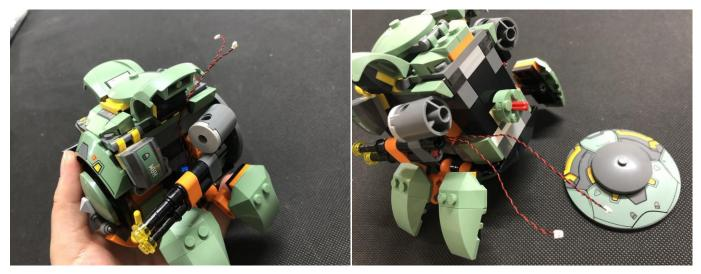
Take the 8-port Expansion Board, connect the cables from the cannons to it
