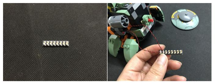
Tuck excess cables, stick the 8-port Expansion Board to the following place with the adhesive squares
