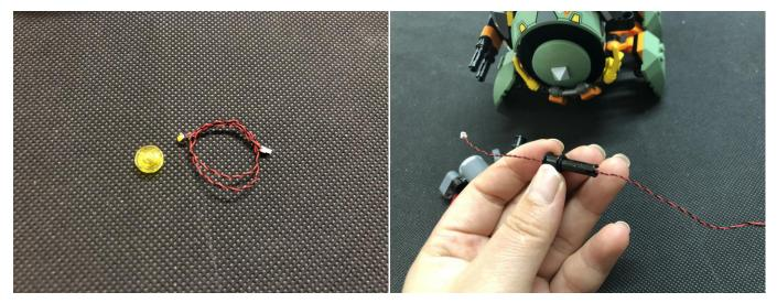
Pull the cable out till the light is placed against the hole, secure the light with the trans yellow piece.
