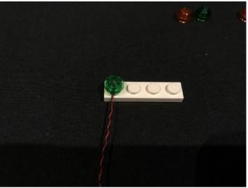
6.) Repeat the previous step to install another 3x Flashing White 15cm Dot Lights to the remaining studs on the 1x4 plate.
