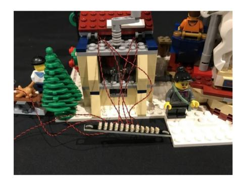
22.) Pull the 30 cm Connecting Cable from the right side over and connect this to the 12-port Expansion Board.
