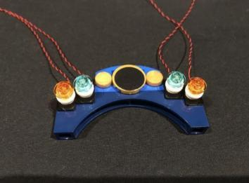
19.) Lift the roof of this stand up and then group the 2x Flashing Dot Light cables from each side together before threading through the inside space that leads to the back side. Thread the cables all the way through and then reconnect the top section.
