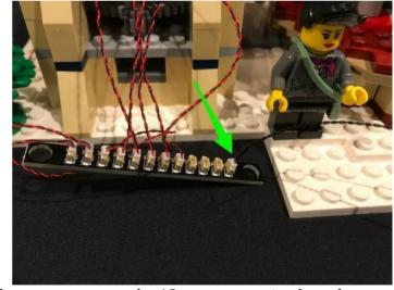
23.) Take the AA Battery Pack and connect it to one of the spare ports on the 12-port expansion board.
