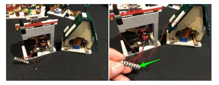
Using 2x Adhesive Squares, mount the expansion board to the base of the Chicken Stand as positioned below:
