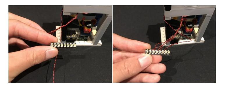
10.) Take the 30cm Connecting Cable and connect this to one of the spare ports.
