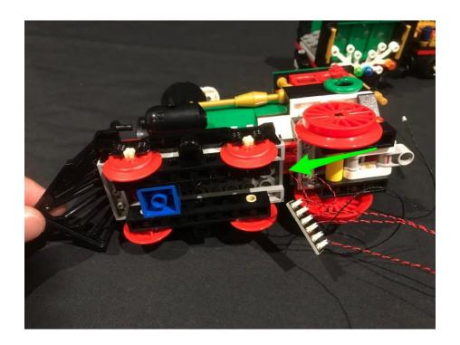
Using 2x Adhesive Squares, stick the expansion board underneath the train in the below position. Neaten all the cables and secure them underneath the back wheels section.
