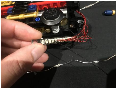
18.) Take a 15cm Connecting Cable and connect it to the next available port along the expansion board then mount the expansion board underneath the carriage in the below position using 4x Adhesive Squares. Neatly tuck in all the cables by pushing them up to prevent them from hanging down and dragging along the tracks. Turn the carriage back over and connect it to the second carriage.
