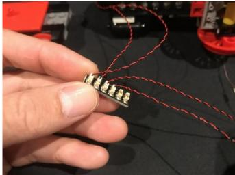
Take a 30cm Connecting Cable and connect one end to the next available port on the expansion board.
