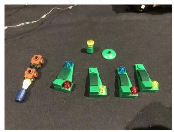
Take a Flashing White 15cm Dot Light and thread the connector side through the top of the green dish. Thread the cable all the way through and then bend the LED on a 90 degree angle so that the LED is facing up.. Place the top section over the LED and then push down and connect it to secure it in place.
