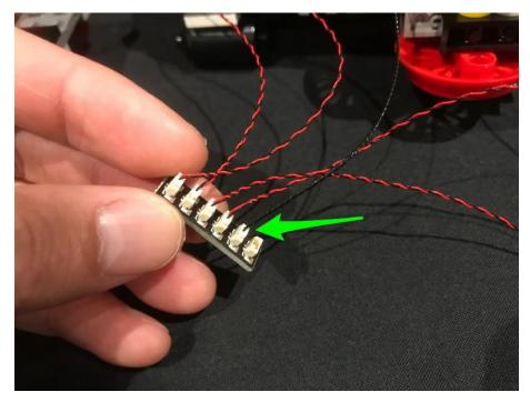
If you have chosen to power using the AA Battery Pack then insert 3x AA Batteries to it and then connect the battery pack cable to the remaining port on the expansion board.
