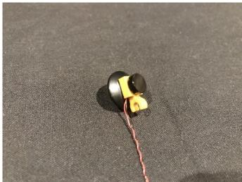
3.) Reconnect both light sections back to the front of the train starting with the top light and ensure both cables are facing down.
