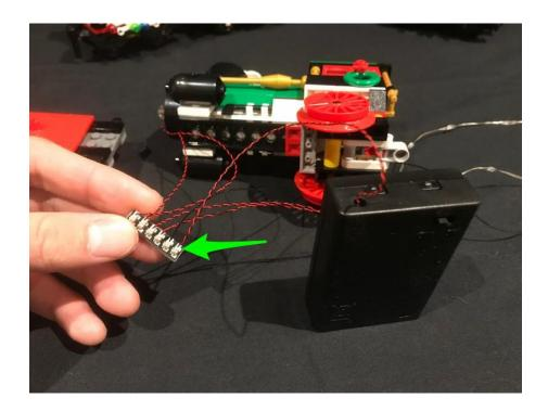
If you have chosen to power using the Vonado Power Functions Cable, then take this cable and connect it to the remaining port on the expansion board (instead of the AA battery pack)
