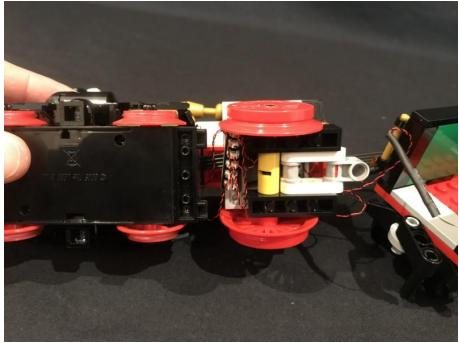
Turn on the battery pack (or connect the power functions cable to power pack) and test that all lights connected are working OK.
