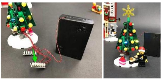
15.) Disconnect the Battery Pack cable from the expansion board and connect one end of a 50cm Connecting Cable to it instead. Take 2x Adhesive Squares and stick one to each side of the dark grey brick at the bottom of the christmas tree.
