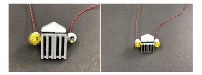
2.) Flip this front section over then take the cable from the right side and fold it over to the left side before reconnecting this section back to the front of the vehicle. Ensure that both cables are laid toward the left.
