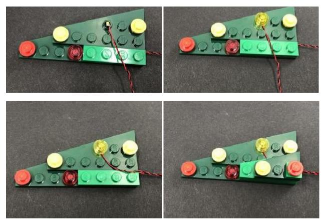
Reconnect this section to the opposite side of the tree where you reconnected the first side section.
