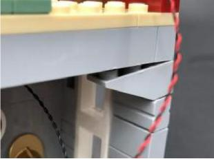
Bring the cable from the lamp down the side of the building and slip it through the gap in between the far right stud. Pull the cable down from the inside to eliminate any excess cable, then connect the Dot Light to the 8-port Expansion Board underneath. Connect up the AA Battery Pack to the expansion board again and turn it ON to test the lamp is working OK.
