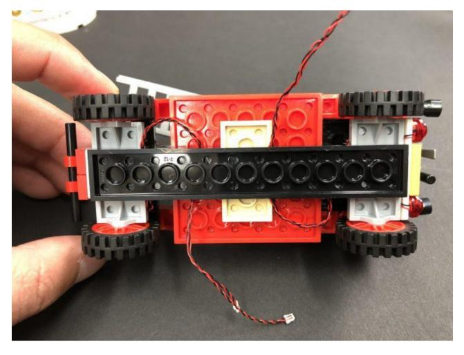
The headlight cables should be laid out toward the left side of the truck and the tail light cables should be laid out toward the right side.
