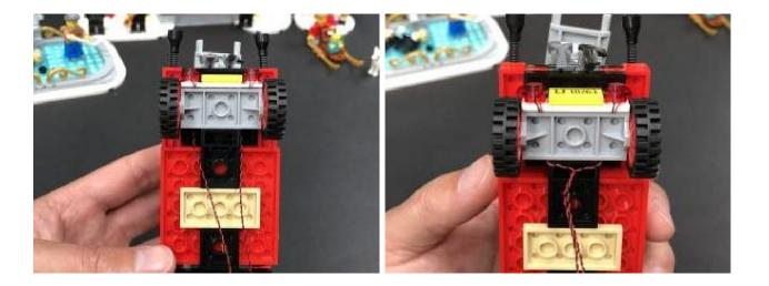
Continue to wind the cables around each other all the way to the ends, then repeat this step to twist/wind the cables from the headlights.
