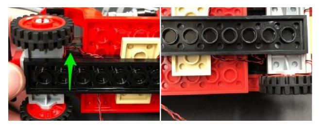
7.) Take a 6-Port Expansion Board and connect all four Dot Light cables to it. Take 2x Adhesive Squares and stick them to the flat side of the expansion board, then mount the expansion board underneath the truck in the following position
