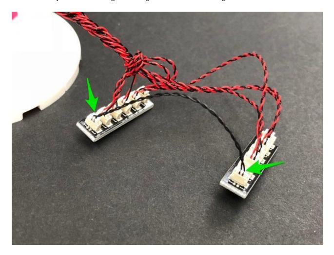
Take the AA Battery Pack and insert 3x AA Batteries to it. Connect the battery pack cable to a spare port on the 6-port expansion board, then turn the battery pack ON to test the christmas tree lights are working OK.
