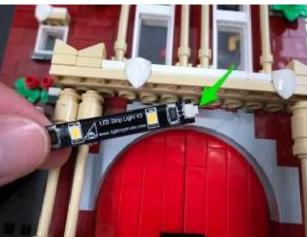
18.) Take a 15cm Connecting Cable and connect it to the Strip Light's left port then using it's adhesive backing, stick the strip light underneath the roof just above the front door as shown below:
