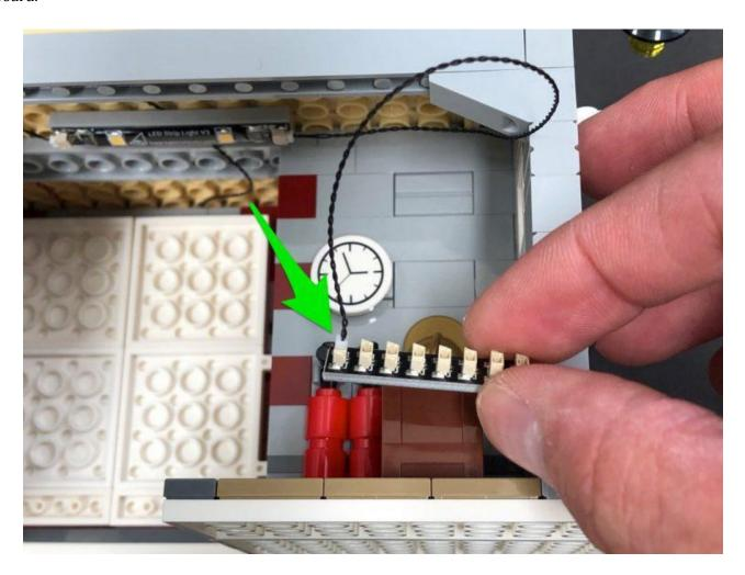
Connect up the AA Battery Pack, the 50cm Connecting Cable from the Ice Rink, and the two Dot Light cables from the lamp post to the 8-Port Expansion Board. Turn the Battery Pack On to test that all lights installed so far are working OK
