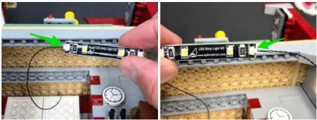
Mount the Strip Light underneath the roof inside the ground floor as shown below. Ensure the newer 15cm connecting cable is facing the right side. To eliminate excess cable in between the two strip lights, loop the cable and tuck in, underneath the strip light.
