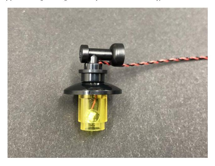
Important Note: Do not forcefully push the tap piece as this may break the cable. The dot light should push down slightly as the tap piece is reconnected.
