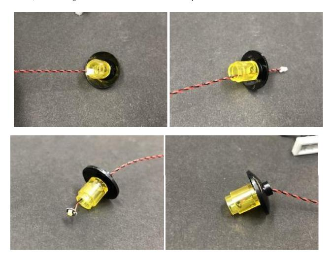
Carefully reconnect the lamp back to the bracket piece but do NOT forcefully push the bracket piece all the way down otherwise it may snap the dot light cable, instead, leave the bracket piece about half a centimetre out.
