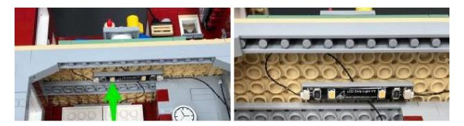
20.) Take the other end of the 15cm Connecting Cable and connect it into the end port on an 8-Port Expansion Board.
