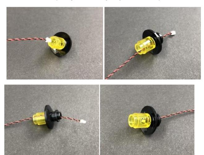
Carefully and slowly reconnect the black tap piece to the top ensuring the dot light is facing the left side of the lamp (This is so the light is shining the correct way when reconnected to the lamp).
