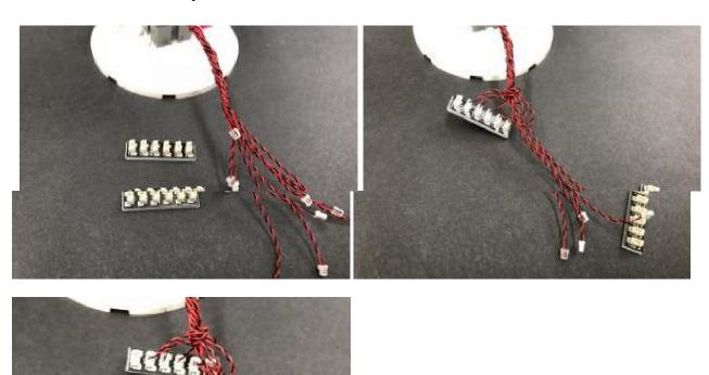
Connect the two expansion boards together using another 5cm Connecting Cable.
