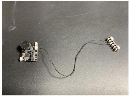
Take a 5cm connecting cable, a 12-port expansion board, connecting them together as per below (in the following picture, we only use the 8-port expansion board for demonstration)
