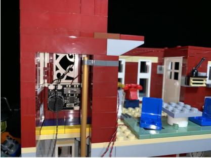
Connect the cables of the lights in the left room to the 6-port expansion board
