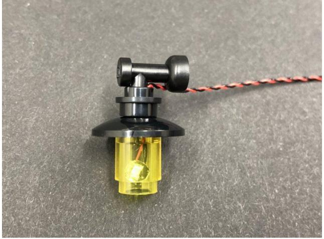
Note: do not force to reconnect the black piece for it may break the cable Thread the connector through the following 1x1 brick, remove the 1x1 round plate, pull the connector out from the bottom of the brick. Pull the connector all the way out before reconnecting the lamp
