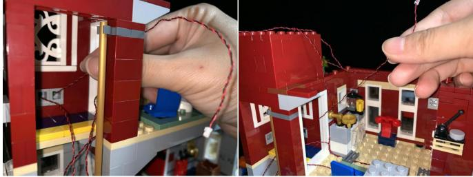
Take a 6-port expansion board, stick tapes at both sides, connect all the 4 cables inside the room to it. Tuck excess cable on the board
