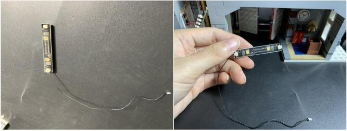
Connect the strip to the roof, then, connect it to the 12-port expansion board
