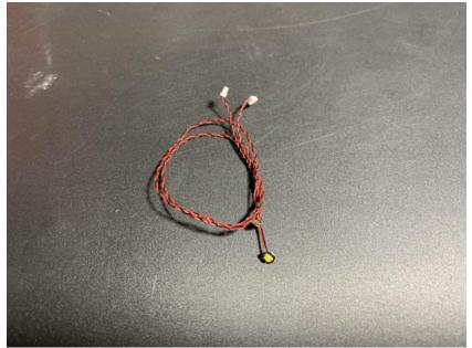
Thread the connector through the hole on the gray piece, pull it out till the light is facing up, then, secure the light by placing the trans yellow piece over it. Repeat this step to install another dot light
