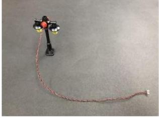
Connect the lamp post back to the base, place the cables underneath in between studs
