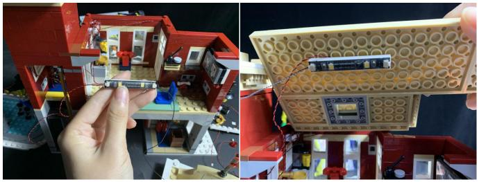
Pull the 15cm connecting cable to the left, connect it to the 12-port expansion board
