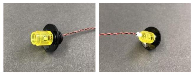
Reconnect the 2 lamps back to the lamp post, group the 2 cables together at the back
