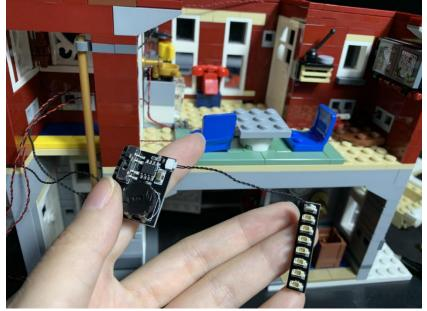
Secure the Multi-Effect Board at the following place by using the tapes
