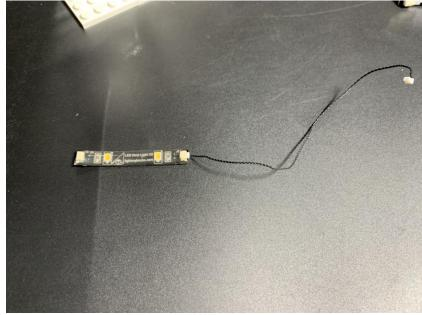
Stick the strip light under the roof of the door, thread the 15cm connecting cable through the door to the back
