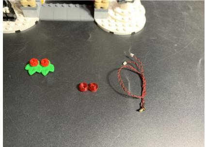
Thread the connector through the green piece, pull till the light is facing up, secure the light by connecting the trans red piece over, then, reconnect the red flower piece.
