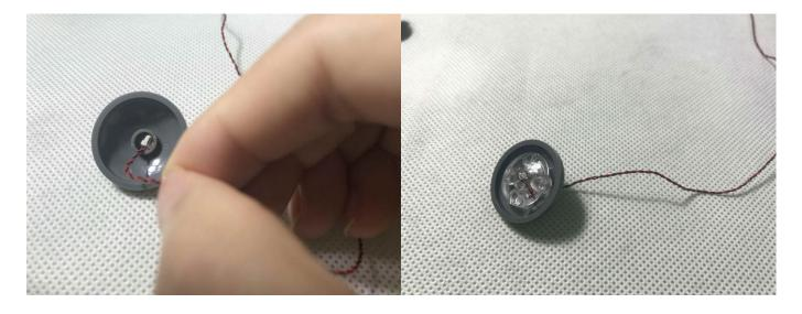
Press the eye part back to the original position. Note: Due to the thin wire, please be careful not to use brute force during installation to avoid tearing and breaking.
