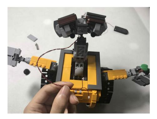
Remove the gray base plate from the neck of the robot, press the cable against the stud gap, and install it back into the gray base plate. Note: In order to ensure that the neck can flex normally, the line should not be pressed too tightly, and the slack should be adjusted appropriately.
