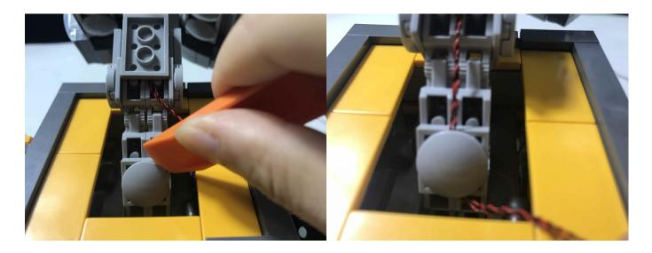
Pass the plug through the gap in the back of the neck and pull it out of the stomach
