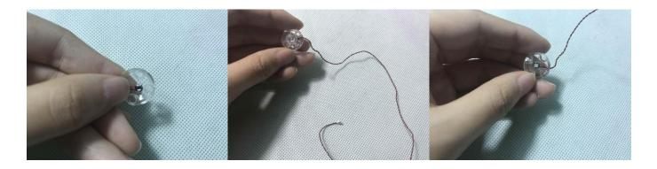
Remove the right side of the robot head, remove the black piece, and replace it with the transparent piece installed.
