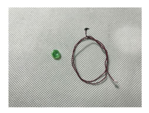
Disconnect the green and brown parts, with the light-emitting side of the Dot Light facing up, the cable facing the side with the square groove at the lower end, fixed with a green transparent piece.
