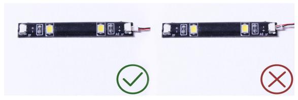
Finally, please pay attention to the positive and negative terminals of the battery when installing the battery case.
