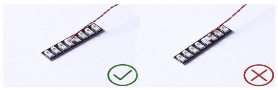
At this point, use the tweezers to straighten the bentpins.
