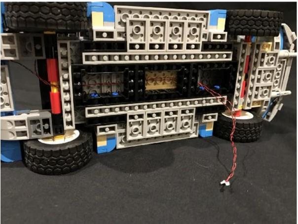
6.) Repeat the above process to install another 2 dot lights with 30cm cablesto the left section of the front of the car.
