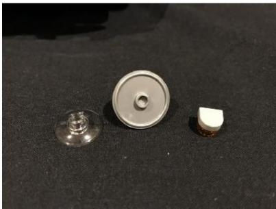
2.) Take one of the dot lights with 30 cm cable and place the LED component part directly over the stud of the headlight. Ensure it is facing the correct way up and then secure it in place by reconnecting the trans dish piece over the top.
