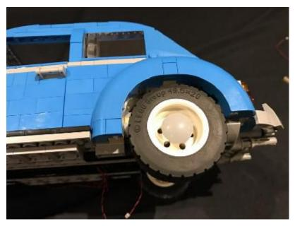
14. ) Pull the cable from the tail light down from underneath the car and then connect this to the next available port on the expansion board.
