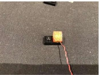
Repeat this step to install another White 30cm Dot Light to this section, securing the light in place by reconnecting the triangular trans clear plate. Then repeat this for the next section to install another 2x White 30cm Dot Lights
