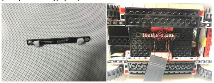
Connect the battery pack to the 12-port expansion board and stick the battery pack to the bottom of the vehicle.
