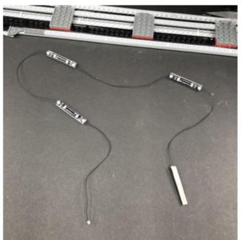
Using the adhesive backing on the end strip light, stick it down toward the right side of the roof section in the following position. Ensure the other components are on the left side.
