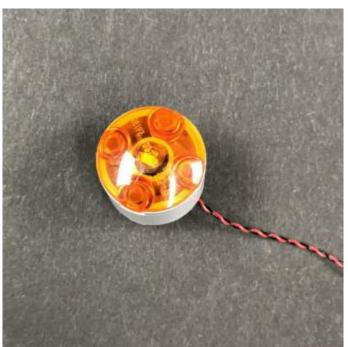
Turn the piece over and reconnect the dark grey round plate ensuring the cable is laid in between the studs.
