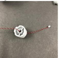
Slightly bend the Dot Light so that it is directly facing upward before pushing it down and reconnecting the trans orange plate over the top.
