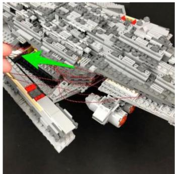
Take the seven cables from the centre jet section and connect them to an 8-Port Expansion Board. Take a 5cm Connecting Cable and connect one end to the remaining port on the expansion board and the other end to one of the OUT ports on the Multi Effects Board (side with 2 ports)
