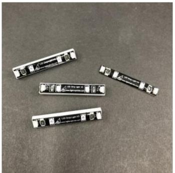
Take a 15cm Connecting Cable and connect it to one of the strip lights that are stuck to a LEGO plate. Take another 3x 15cm Connecting Cables and connect the remaining strip lights together ensuring the strip light that is not stuck to a LEGO plate is on the very end.
