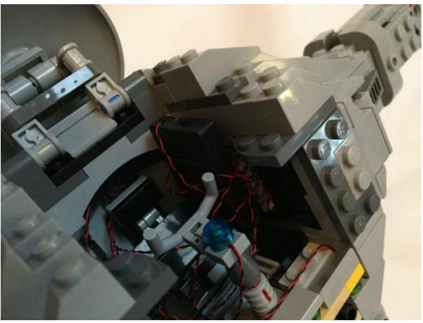
Place the 6 Port Expansion Board into the cavity on the right hand side of the cockpit and slide the Battery Pack down next to it (with the switch facing up towards the hatch).
