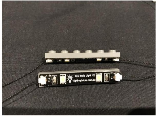
Connect the strip lights to each side of the inside of the tower in below positions.
