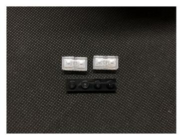
Take 4 warm white dot lights, with lighting part facing up, place the lights to the following places, and connect the trans piece over to secure the lights
