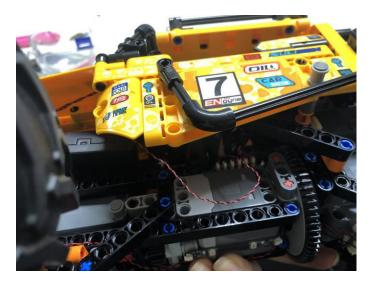
Turn the power on to test if all lights are working OK
