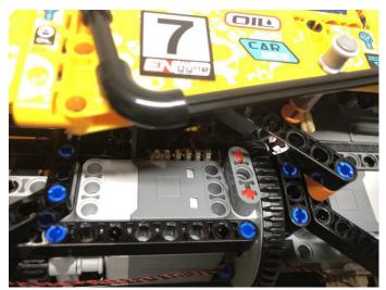
Take a 6-port expansion board, a 5 cm connecting cable, connect the connecting cables to the expansion board
