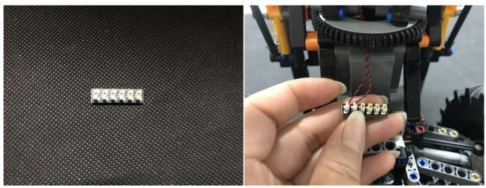
Stick the expansion board to the bottom of the car with the adhesive squares
