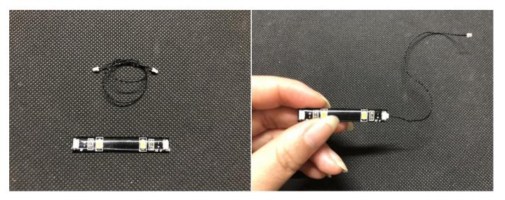
Stick the strip light to the roof of the driver's room, pull the cable down to the bottom as  $\operatorname{per}$  below
