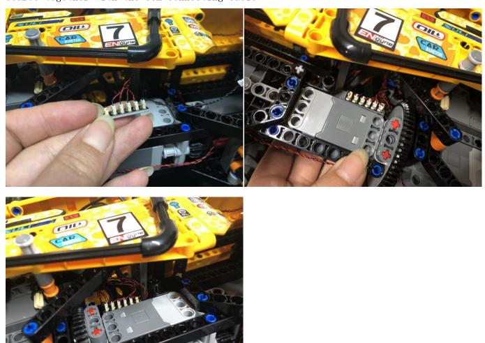
Take a warm white strip light, a 15cm connecting cable, connect the connecting cable to the strip light
