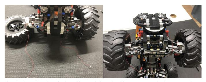
Thread the cable through the following hole and pull it out from the bottom of the car
