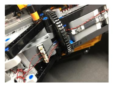
Take a 15cm connecting cable, connect it to the expansion board underneath
