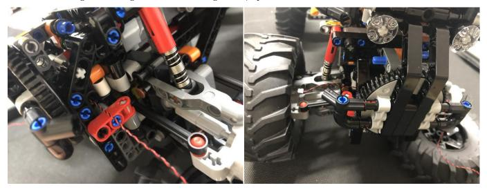
Secure the bolt to the following place, reconnect the tire
