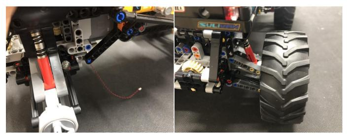
Place the car upright, pull the cable to the bottom of the car, and connect it to the expansion board
