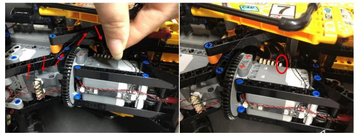
Take a 15cm connecting cable, connect it to the strip light inside the driver's room, and pull it to the back, connect it to the 12-port expansion board
