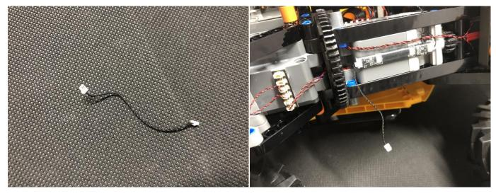
Thread the cable through the following hole and connect it to the expansion board nearby
