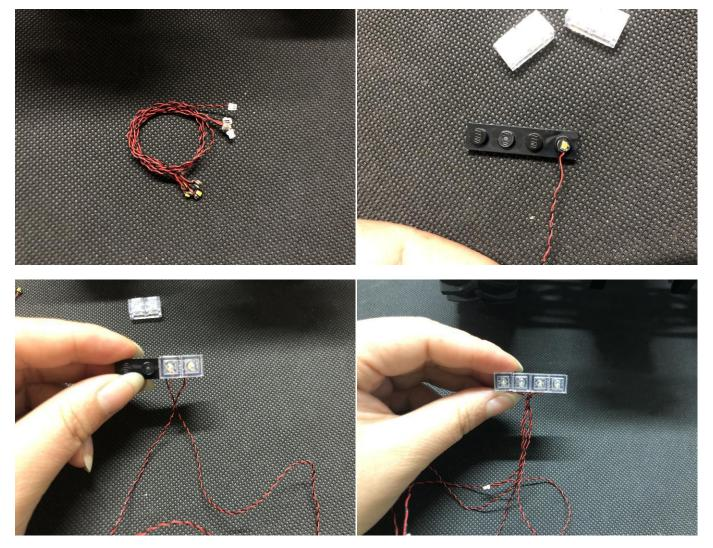
Group the cables together, thread the cables through the following hole as per below
