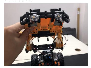
Pull the cables of the headlights backward, thread the cables through the following hole
