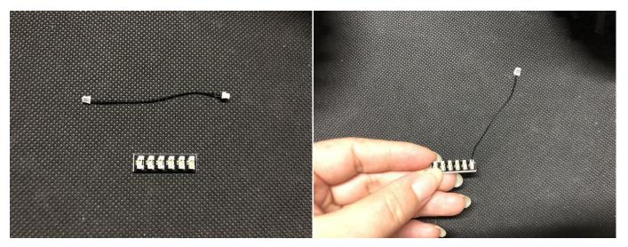
Connect the 4 cables from the other side to the expansion board, connect the 2 expansion boards together with the  $5 \, \mathrm{cm}$  connecting cable
