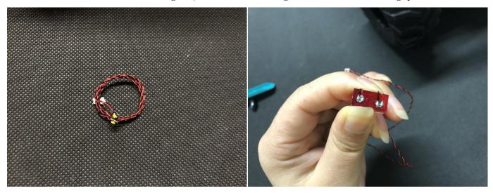
Reconnect the taillights, connect the cables to the expansion board
