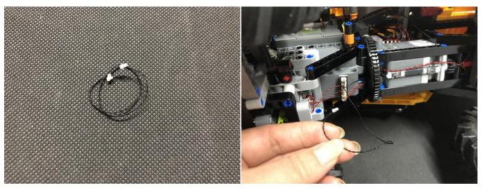
Place the cable as per below to connect the other end of the cable to the following expansion board
