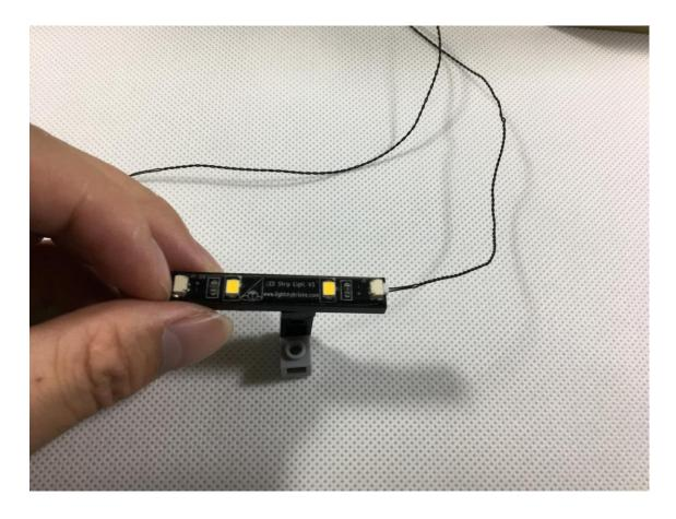
Pay attention to the position of cable. Thread into the small hole of the piece out of the hole below
