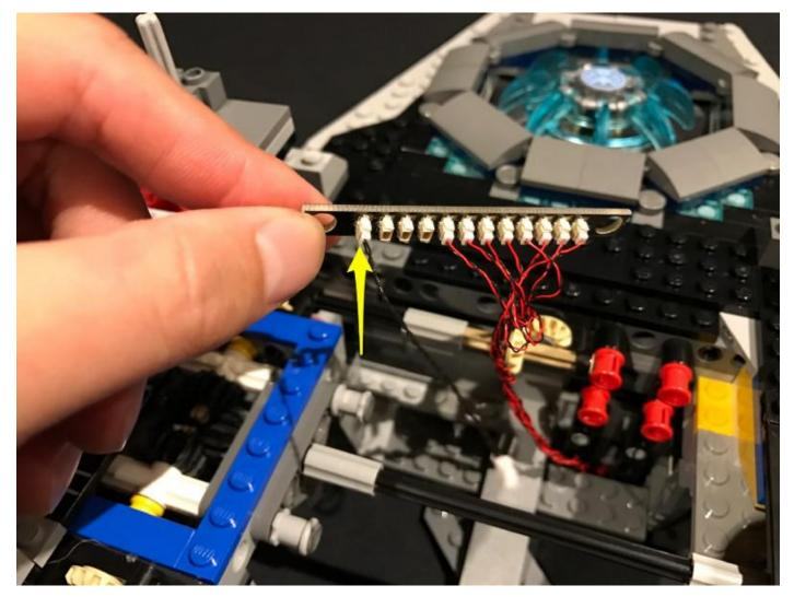
4.) Connect the two 12-port expansion boards (with the other end of each 5cm cable) to the each "output" port on the Multi-Effects Board (side with 2 ports). Take another 5cm connecting cable and then connect it to a 6-port Expansion Board. Connect the other end of this 5cm connecting cable to the "input" port on the Multi Effects Board.
