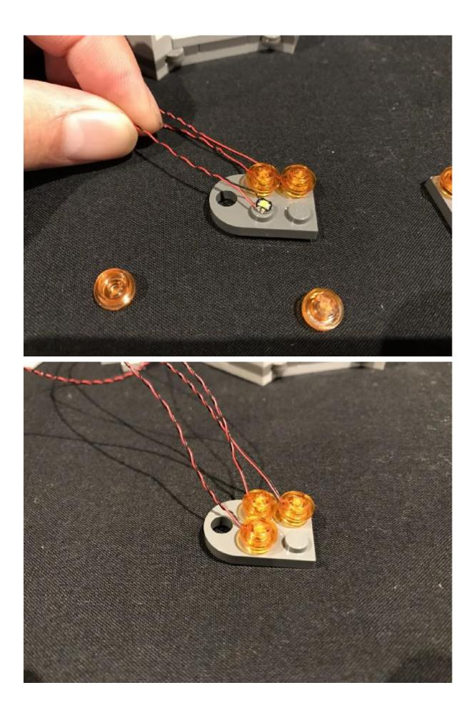
To install a Dot Light to the trans orange plate that connects to the "hole", take another White 30cm Dot Light and then bend it up on a 90 degree angle and the place it inside the "hole" as per below:
