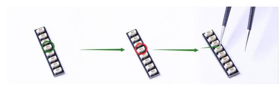
When installing dot lights, make sure they are correctly placed (Yellow LED package is exposed). You can put they either on the top of the studs or between studs.
