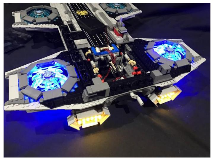
7.) Remove another LEGO road plate and then take another 15cm connecting cable and connect it to the 6-port expansion board. This cable will be used to connect this sections of lights to the front half of the helicarrier.
