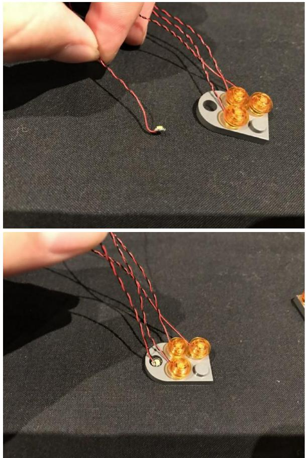
Reconnect the trans-orange plate over the top (upside down) ensuring the cable is facing the same way
