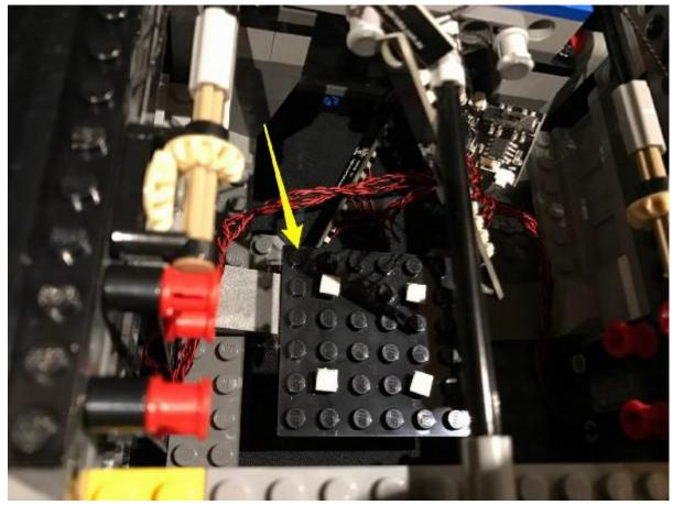
Place the AA Battery Pack on top of the 6x6 plate and secure down ensuring it is well mounted to the plate underneath.
