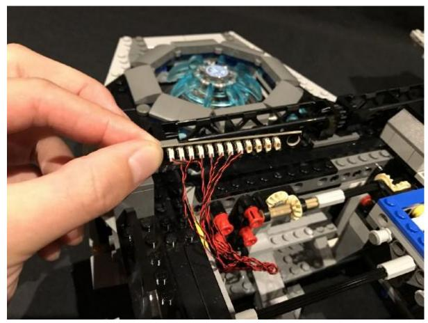
Take a 5cm connecting cable and then connect this to a spare port on the expansion board.
