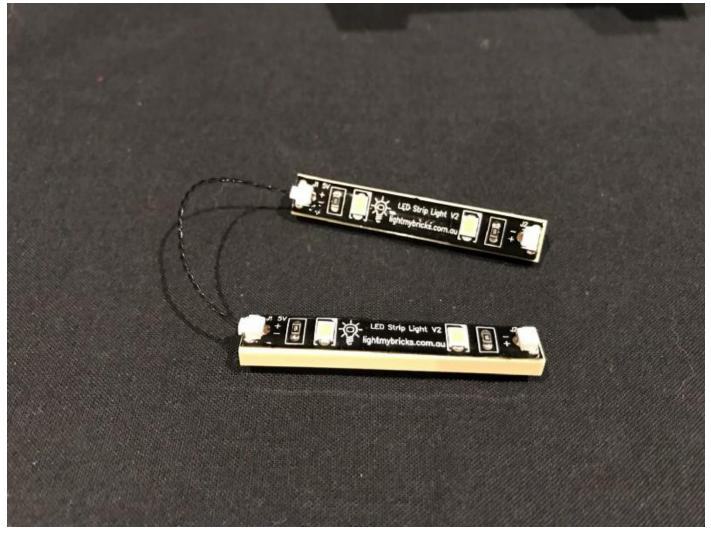
Take the LEGO Road plate section (with logo on the top) and then turn over to allow us to mount the 2x White Strip Lights underneath in the following position. Before mounting strip lights, connect the other end of the 15cm cable from expansion board to one of the White Strip Lights.
