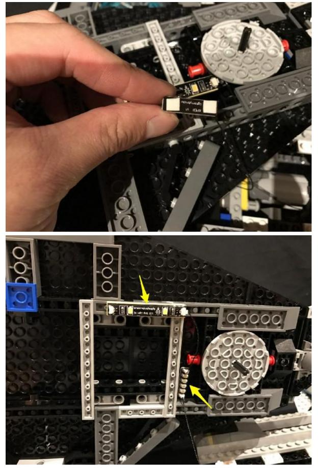
Take the control room section and then place it on top of the helicarrier towards the right and connect both the Dot Light cables from the control room to the 6-port expansion board.
