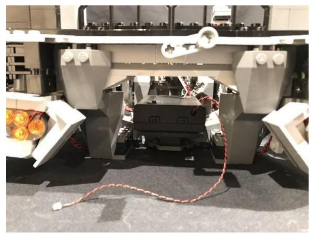
Thread the battery pack cable back inside and then pull up from the inside and then connect it to the 6-port expansion board.
