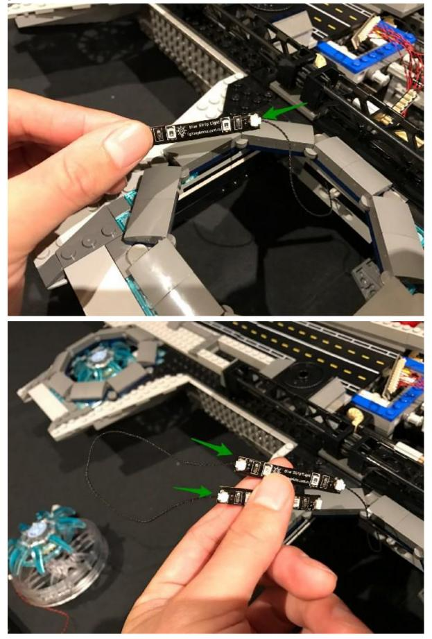
Using the adhesive backing for each strip light, stick them to the sides on the inside of this section.
