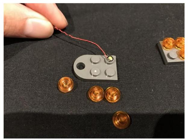
Ensure the cable is facing toward the top left, then secure the Dot Light in place by reconnecting one of the trans-orange plates over the top.
