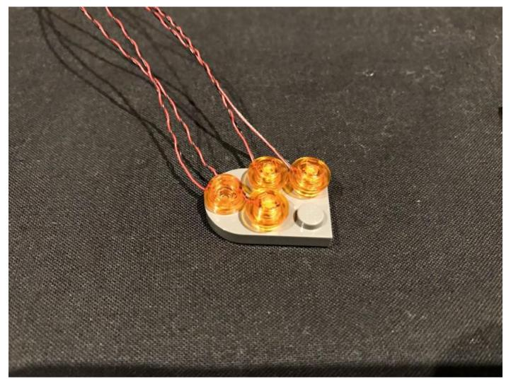
Take all the cables from the Dot Lights we just installed and then twist/wind them together so they form one large cable.
