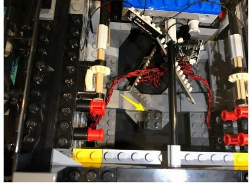
Take 4x adhesive squares and stick them to the following studs on the 6x6 plate, then connect the plate to the 2x2 brick as per below.
