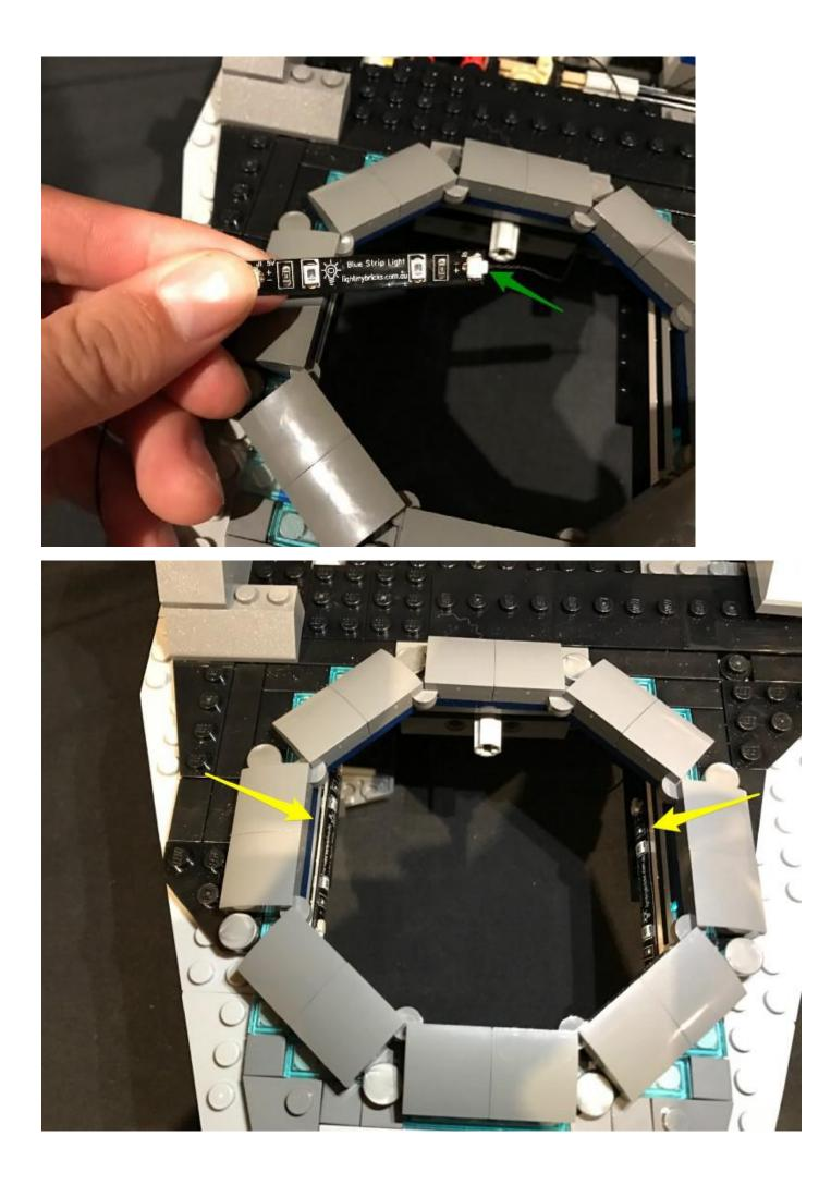
Eliminate excess cable by connecting under LEGO plates and then reconnect propeller.
