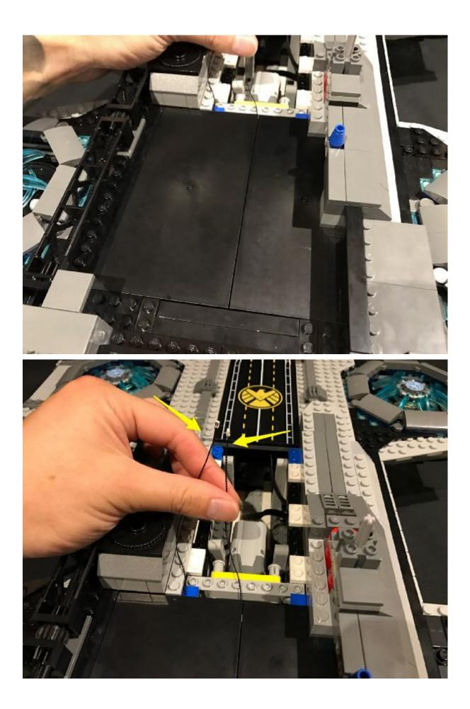
10.) Take another 2x 6-port Expansion Boards and connect each of the 15cm cables we pulled through to one expansion board.
