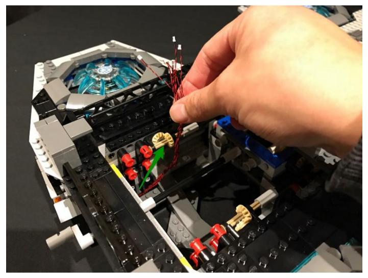
Connect all the cables to a 12-port Expansion Board
