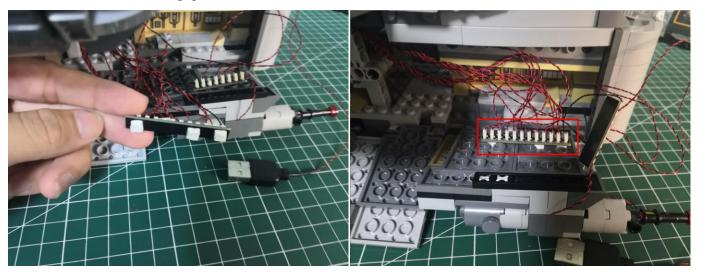
Stick 2 adhesive squares to the back of the 8-port expansion board, stick the expansion board to the following place.
