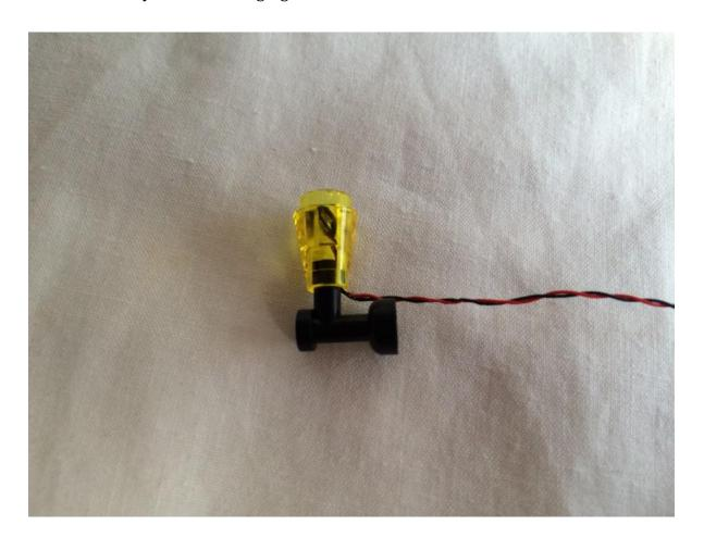
Very slowly, join the transparent yellow cone piece and the black tap piece back together. It is a tight fit and doing this slowly will prevent damage to the wires.
