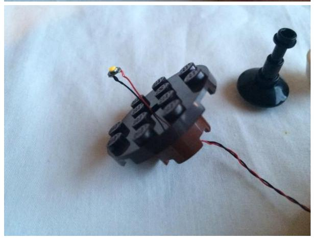
Grab a White Dot Light and feed the LED component end up through the bottom of the round 2 x 2 brick under the table.
