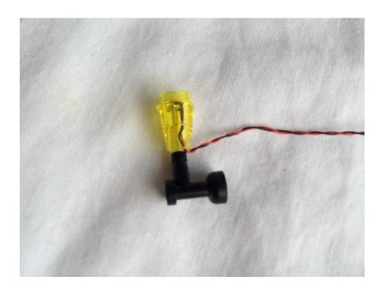
Bend the wire so that it comes out the transparent yellow cone piece at a right angle. Line up the black tap piece to insert back into the transparent yellow cone piece. Have the large round end facing the same way as the wire coming out of the transparent yellow cone piece. In the photos, you can see that they are both facing right.
