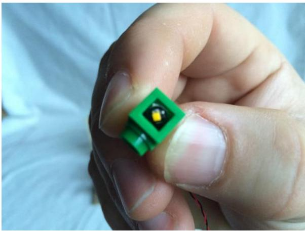
As you continue to pull the LED wire through, try to arrange it so that the yellow LED component is mostly facing outwards from the brick. If it is facing inwards, you may not get the best lighting effect for this piece.
