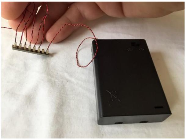
Grab your battery pack and connect it to an available slot on the 8 Port Expansion Board.
