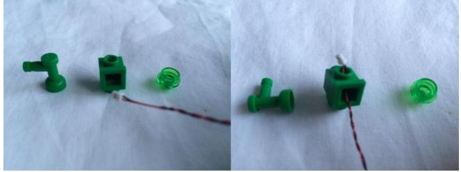
Grab a White Dot Light and feed the plug end through the square opening of the green headlight piece. Get it to exit the green headlight piece through the round opening. Sometimes we need to bend the wires slightly near the plug end of the wire to get it to feed through.
