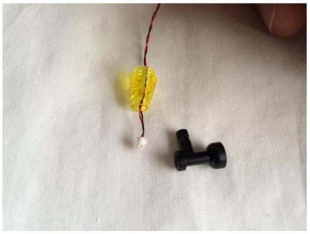
Grab a White Dot Light and feed the plug end through the large end of the transparent yellow cone piece.
