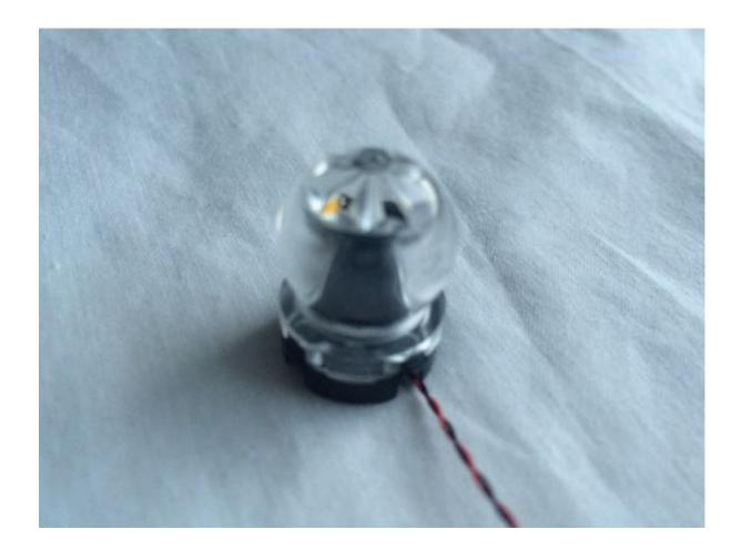
Pull the wires through until the LED component is sitting face up on top of the black 1 x 1 round brick. Replace the transparent clear top piece.
