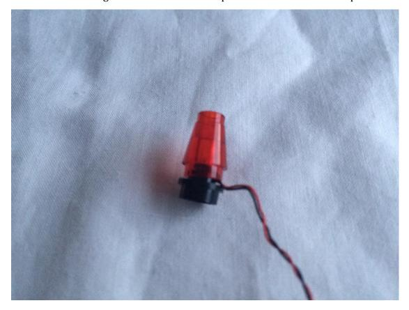
Very slowly, join the transparent red cone piece and the black round plate back together. It is a tight fit and doing this slowly will prevent damage to the wires.
