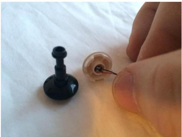
Run enough wire through so that you can rest the LED inside the lampshade with the yellow LED component facing the top of the lampshade.
