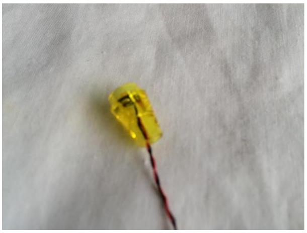
Pull the wires all the way through until the LED is inside the transparent yellow cone piece.
