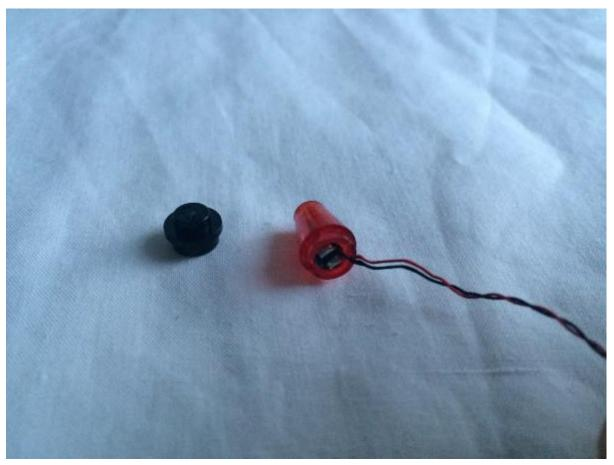
Grab a White Dot Light and rest the LED component end inside the transparent red cone piece.
