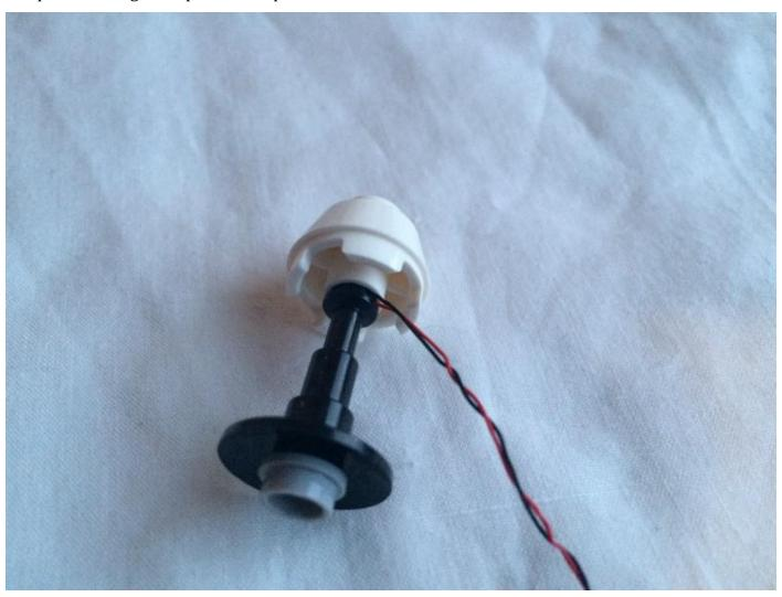
Very slowly, join the stem of the lamp shade and the lamp back together. It is a tight fit and doing this slowly will prevent damage to the wires.
