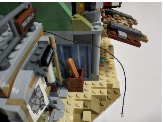
Connect the 15cm connecting cable to the left port of the other strip , stick the strip under the eaves
