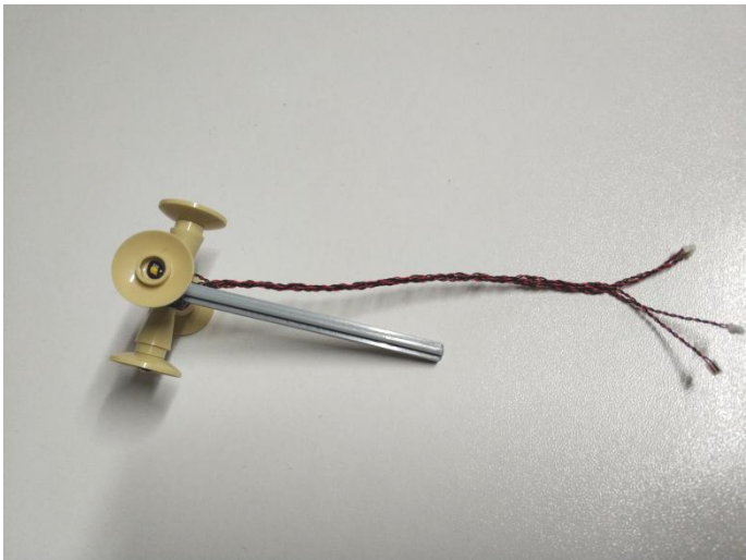
remove the gray round plate, reconnect it, wind the cables around the pole
