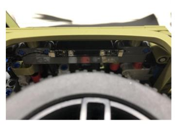
Thread the connecting cable through the following hole to the bottom of the car, and  $\operatorname{pull}$  it backward
