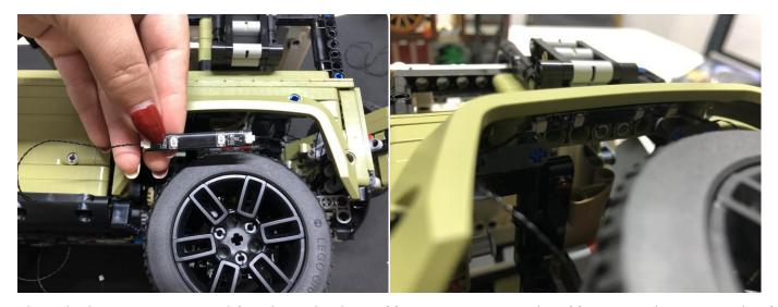
Thread the connecting cable through the following space, and pull it to the front wheel
