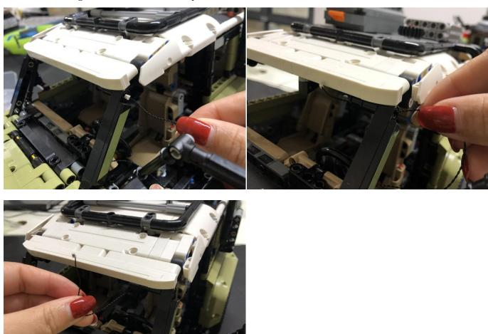
Thread the cable through the hole of the piece above the front seat
