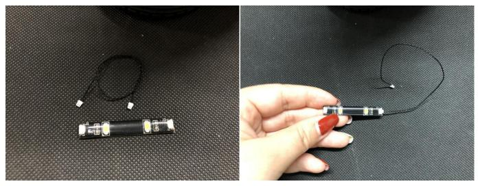
Connect the cable from the roof to the left port of the strip light, stick the strip light to the roof
