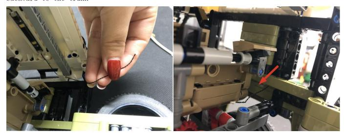
Take a 8-port expansion board, connect the cable to it
