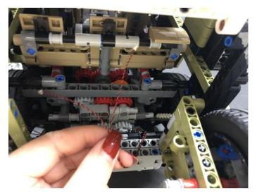
connect the cable to the expansion board
