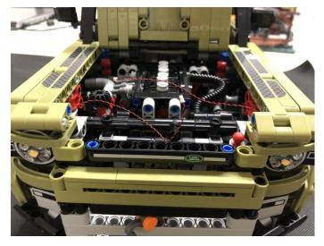
Take a 6-port expansion board, connect the cables of the headlights to it
