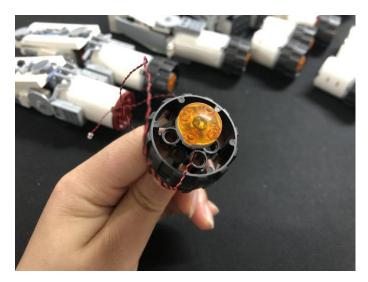
Thread the cable through the black hole before reconnecting the black piece
