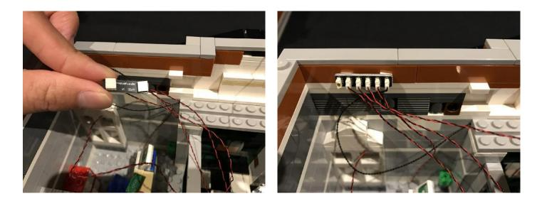
15.) Tidy up excess cables by grouping them together and placing them in the middle. You can secure them and prevent them from dangling down by using tape or a spare LEGO brick to connect over them. The key here is to ensure these cables are not visible from the outside looking in through the front windows.
