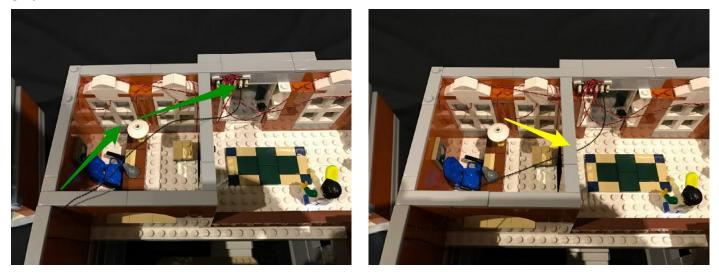
24.) We can now test the lights we have installed so far. Take the battery pack and connect the battery pack cable to the expansion board on the second level. Turn on to verify all is working OK
