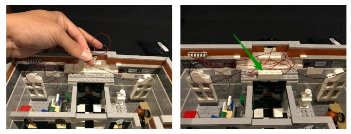
16.) Now is a good time to test our current lights we have installed so far. To do this take the Battery Pack and insert 3x AA batteries into it. Plug the battery cable into the spare port on the expansion board and then turn "ON" to verify all the lights at the front are working.
