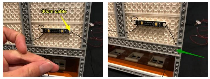
22.) Thread the other end of the 30cm cable into the space that leads above. Turn the second floor over and pull it up from underneath.
