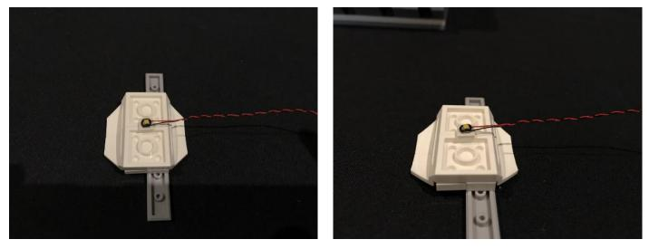
Reconnect this section back ensuring the cable is laid behind then reconnect the grey plate we removed earlier. You should be able to see the LED component peaking out if you look from below up.
