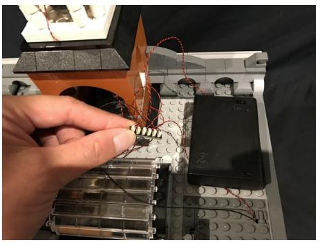
Mount the expansion board to the following position on top of the roof using 2x adhesive squares.
