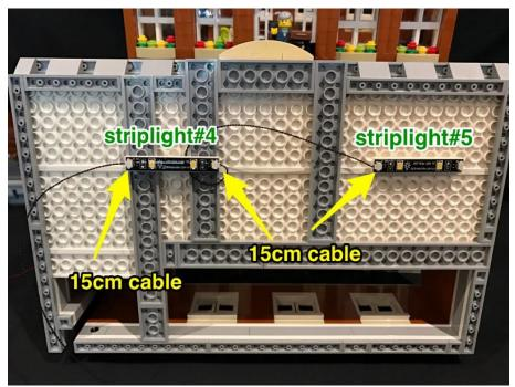
27.) Connect a 30cm connecting cable to the right port on striplight#5 and then thread the cable up into the space which leads above. Ensure you secure this cable underneath the grey plate as shown below:
