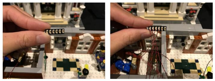
To eliminate excess cabling, wind the cables around the expansion board as shown below and then mount the expansion board to the following position on the wall inside the second floor using 2x adhesive squares.
