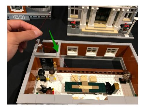
26.) Turn this level over and connect/stick another two LED Strip Lights(striplight#4 and striplight#5) to the following positions. Connect them together using another 15cm connecting cable and connect another 15cm connecting cable to the left port on striplight#4
