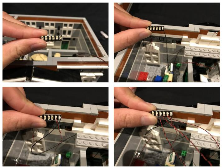
Use 2x adhesive squares to mount the expansion board to the inside of the front of the wall as shown below.
