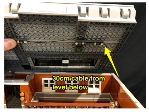
Thread the other end of the Dot Light cable from the window up the through the doorway (through the same hole as the connecting cable) and then pull it all the way up from the top before closing the door again.
