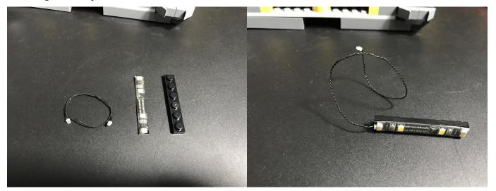
Install the strip at the back of the display board, ensure you place the cable in between the studs
