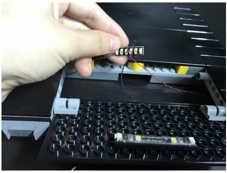
Take the battery pack, insert batteries to it before connecting the battery cable into the port on the expansion board. Stick the adhesive tapes at 2 sides of the expansion board
