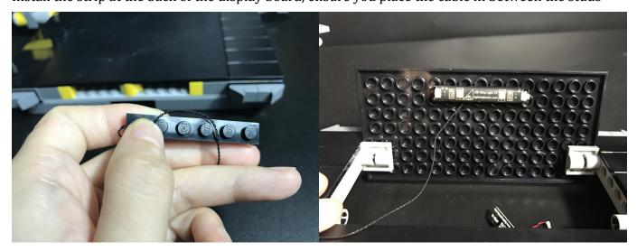
Connect the other end of the 15cm connecting cable to the expansion board
