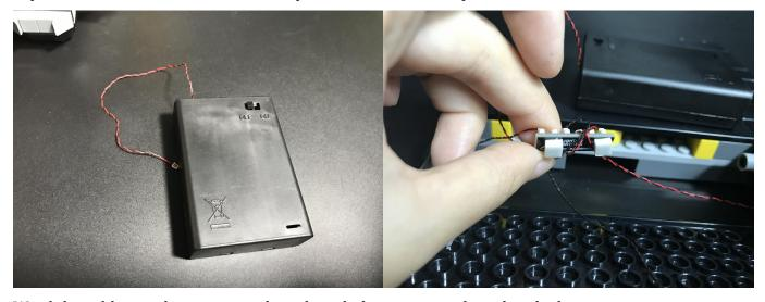
Wind the cables on the expansion board, stick the expansion board at the base.
