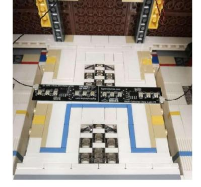
40.) Take the entire middle section of the Taj Mahal over the ground koor and then locate the other end of the 30cm connecting cable from the 8-port expansion board and then connect it to one of the 6-port expansion boards on the ground koor below.
