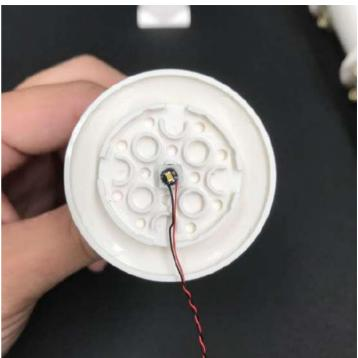
4.) Reconnect the roof ensuring the cable from the Dot Light is facing one of the corners, then disconnect the bottom of the tower from the below position:
