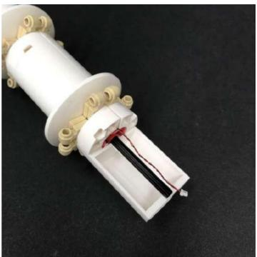
11.) Take a 6-port Expansion Board and connect a 30cm Connecting Cable to a spare port. Connect the end of the Dot Light Cable from the tower to the expansion board and then tuck both components inside the wall section of the tower while ensuring the 30cm connecting cable is laid down the middle of the wall piece.
