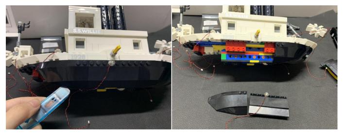
Place the cable of the light from the black piece underneath in between studs, reconnect the following pieces
