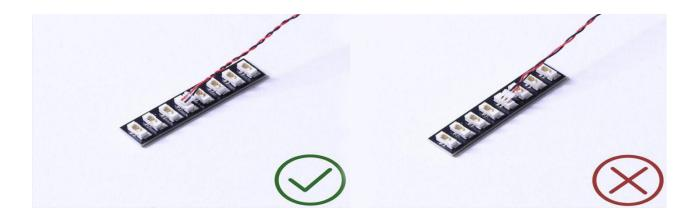
At this point, use the tweezers to straighten the bentpins.
