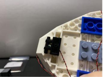
Take the Remote Control Switch Board, the USB Power Cable. Connect the 30cm connecting cable of the warm white light to the remote control switch board
