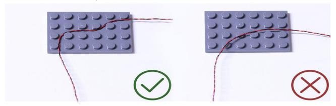
Insert the connectors to the ports.
