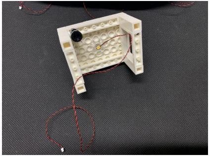
Remove one side of the window pieces, thread the connector of the light through the following holes on the piece, pull it out
