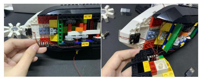
Take a 5cm connecting cable, connect to the 6-port expansion board at the head of the boat, connect the other end of the cable to the remote control switch board. Place the board to the following position
