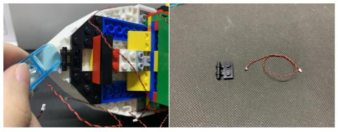
With lighting part downward, place the dot light at the hole on the black plate. Reconnect the black plate back to the head of the boat, from the bottom of the boat, pull the cable backward
