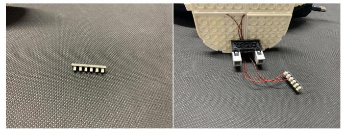
Take a 30cm connecting cable, connect it to the 6-port expansion board. Connect the other end of the cable to the remote control switch board. Stick the expansion board to the back of the board
