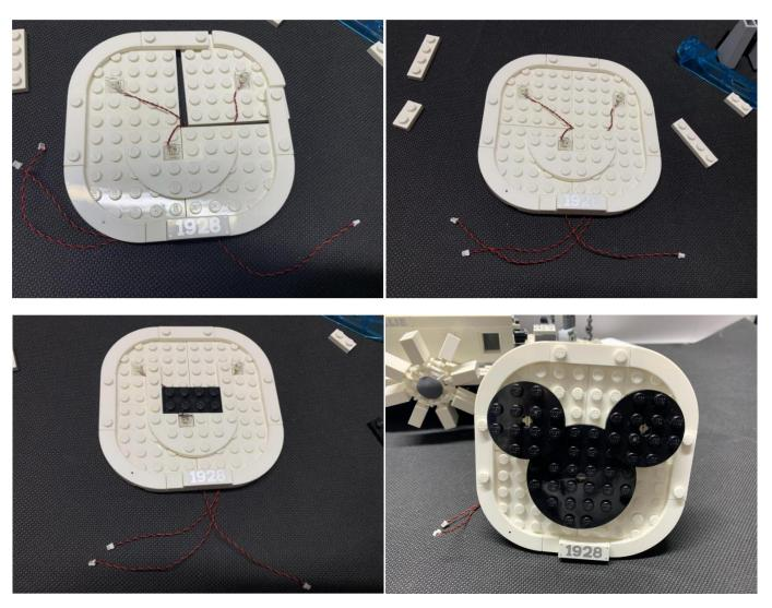
Take a 6-port expansion board, connect the cables of the lights to it
