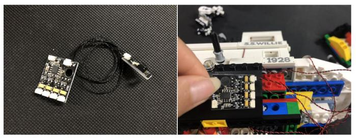
Take the 8-port Expansion Board, connect a 30cm connecting cable to it
