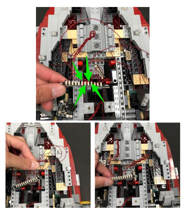
33.) Take the AA Battery Pack and connect the cable to one of the ports on the 12-port Expansion Board. Turn the power 'ON' to verify all lights are working OK
