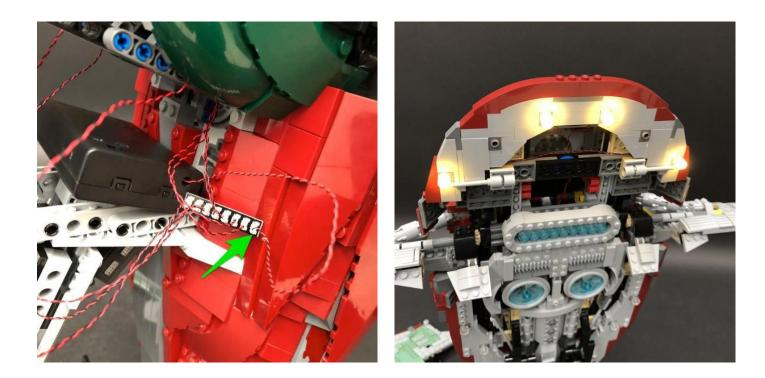
13.) Disconnect the AA Battery Pack and connect a 5cm Connecting Cableinto the expansion board.
