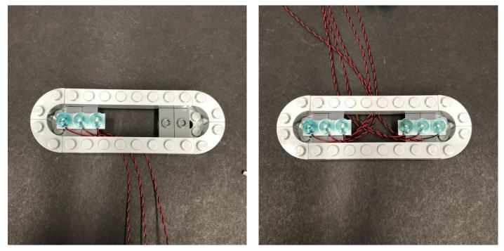
Group the three cables from each side and then reconnect this section back to Slave 1. Ensure that the cables from each side are neatly laid facing down as per below:
