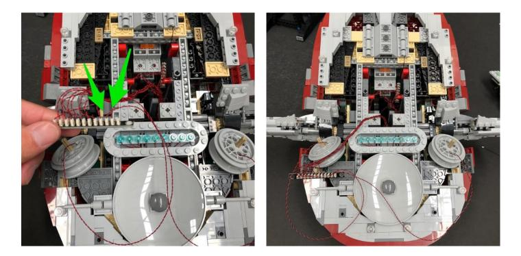
22.) Take a 5cm Connecting Cable and connect one side to the remaining port on the 12-port Expansion Board. Connect the other side to one of the OUT ports on the Multi Effects Board (side with 2 ports)
