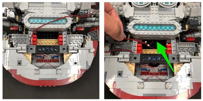
Pull the four cables out from the front side of Slave 1and then connect them to the 8-port expansion board from step 7.
