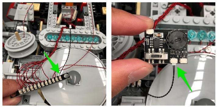
Setup and test the effects of the Multi Effects Board by connecting the AA Battery Pack to the IN port (side with 1 port). Turn 'ON' the battery pack and then set the switch to the left for the "Pulse" effect. Turn the wheel to adjust to the slowest speed. Alternatively, set the switch and adjust the speed to your desired effect.
