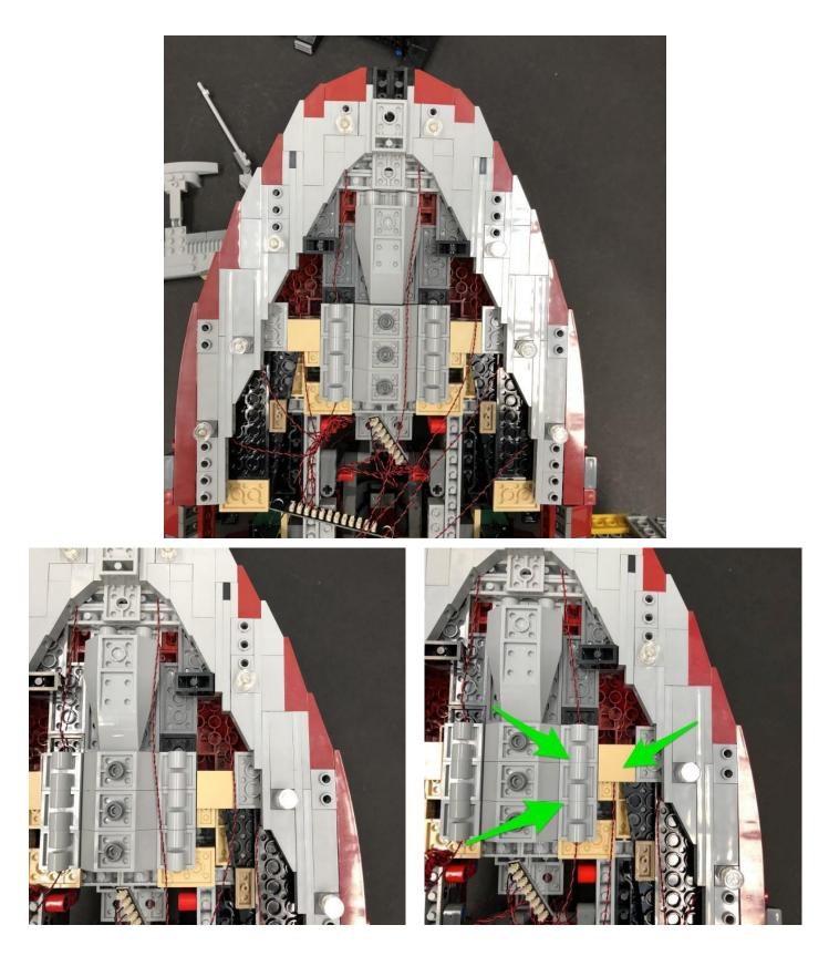
32.) Connect the four Dot Light cables from the right side to the next available ports on the 12-port expansion board then neaten up cabling by grouping and twisting the cables together.
