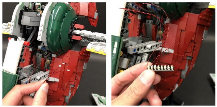
Take this time to test the lights we have installed so far by inserting 3x AA Batteries to the AA Battery Pack and then connect the battery pack cable to a spare port on the expansion board. Turn 'ON' to verify all is working OK.
