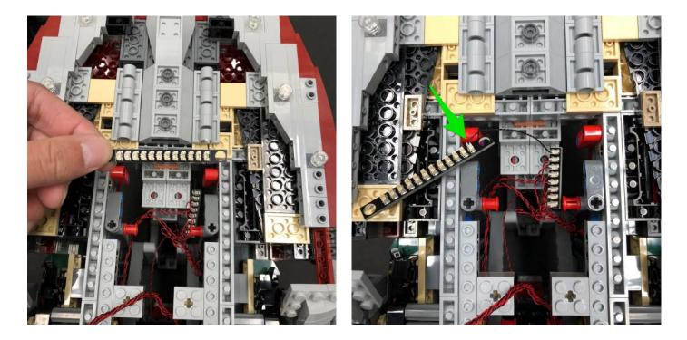
25.) Connect the other side of the 5cm connecting cable from the multi effects board to the far left port on the new 12-Port Expansion Board
