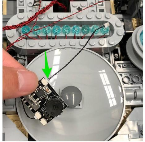
24.) Take the remaining 12-Port Expansion Board and then connect to the far right port, the other end of the 5cm cable from the 8-port expansion board from step 7.
