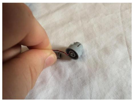
Gently replace the technic rod into the hole where the LED is. It will be a tight fit so you need to do it slowly to prevent damage.
