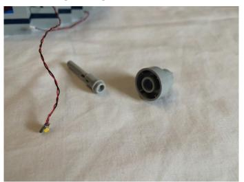
We are going to place the Dot Light inside the larger round piece making sure that the LED faces away from the hole we will put it in to. Gently bend the wires until it resembles the image below:
