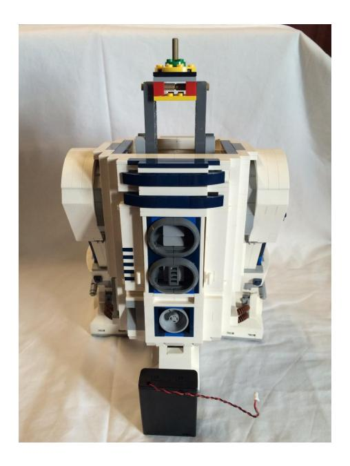
Turn R2 around and sit the battery pack horizontally inside his body with the switch on the high side and facing back towards you.
