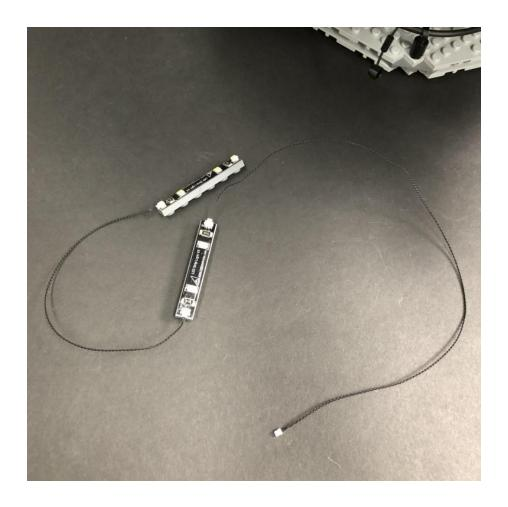
Connect the other end of the 15cm connecting cable from the room on the right (yellow crane room) to the strip light with a free port. Mount the two strip lights to the top of this room ensuring the spare end of the 30cm connecting cable is facing the inside.
