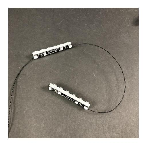
Connect the other end of the 15cm Connecting Cable from the Red Strip Light to the Blue Strip Light with a free port.
