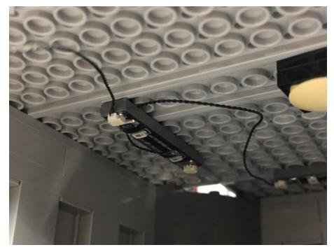
27.) Hide the cable between the Blue and Red Strip Light by laying it underneath the floor. Use the LEGO removal tool to create a gap to slip the cable underneath ensuring the cable is in between studs, then reconnect the floor. Tuck in any remaining excess cable by pushing it up to secure between connectors.
