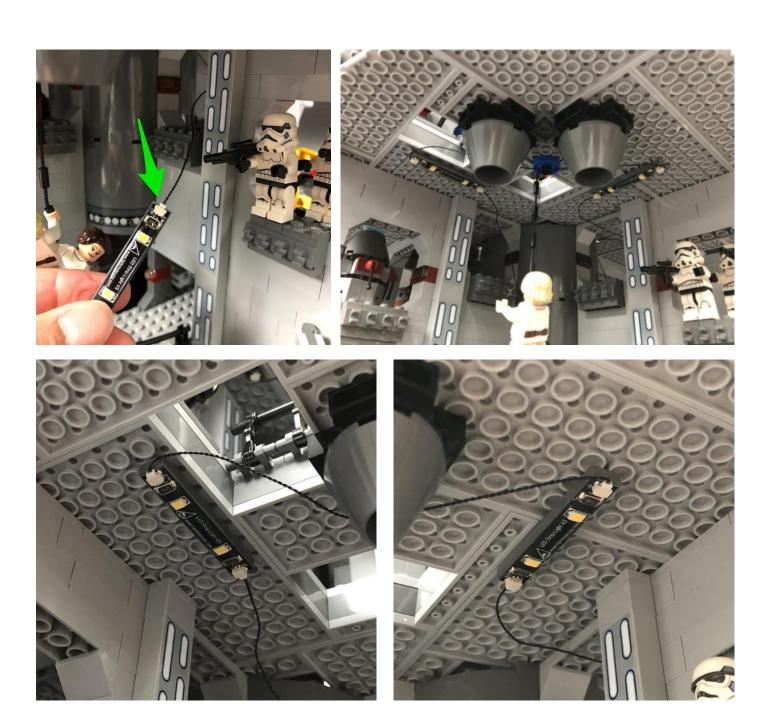
43.) Thread the 30cm connecting cable down through hole on the left which leads the bottom space where the 50cm connecting cable from step 34 is
