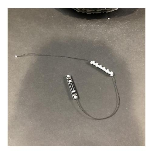
Take the other end of the 15cm connecting cable from the Blue Strip Light and connect it to the Red Strip Light that has a free port.
