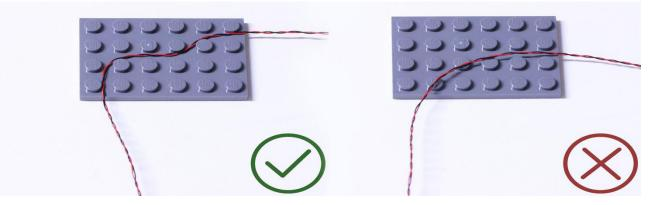
Insert the connectors to the ports.
