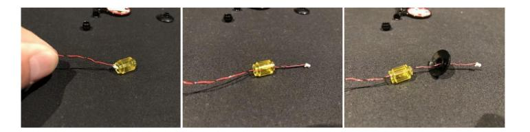
Pull the cable all the way through from the top until the LED component is right up against the inside of the trans yellow brick, then reconnect the 2 pieces (black dish and trans yellow brick) together.
