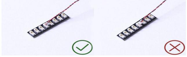
At this point, use the tweezers to straighten the bentpins.
