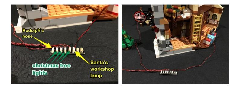
9.) To eliminate excess cable from Santa's Workshop lamp, wind it around the expansion board a few times and then secure the expansion board to the base of the building using a self adhesive square as per below:
