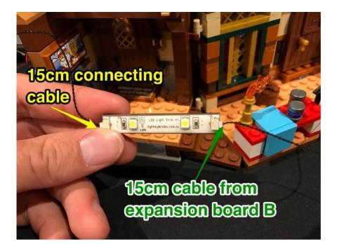
19.) Connect/Stick this strip light underneath the second koor of Santa's Workshop in the below position and then connect the other end of the 15cm cable on the left to the next available port on Expansion Board A.
