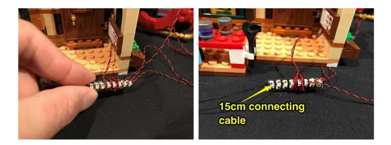
18.) Take the LED Strip Light and connect the 15cm cable from expansion board B to the port on the right of the strip light. Take another 15cm connecting cable and connect it to the port on the left.
