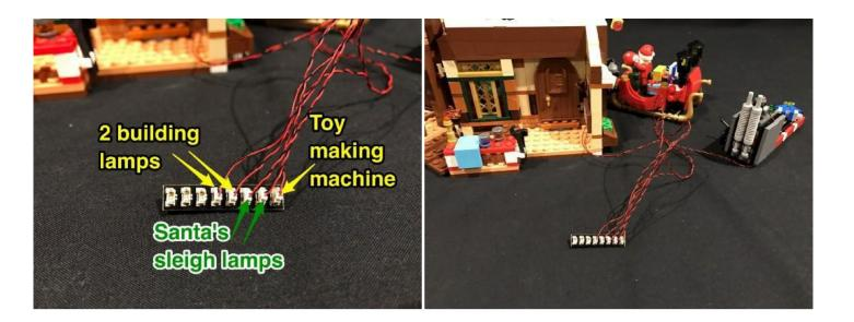
17.) Wind the cables from the building lamps around the expansion board a few times, then connect a 15cm connecting cable to the port furthest to the left.
