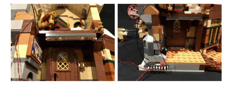
20.) Lay the 15cm cable between expansion boards A and B underneath the desk ensuring the cable is laid neatly in between studs. Stick Expansion board B to the side of the orange base using provided adhesive squares.
