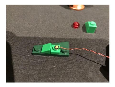
Secure the Dot Light in place by reconnecting the trans red round plate directly over the top, then reconnect the light green brick next to it ensuring the cable underneath is laid in between studs.
