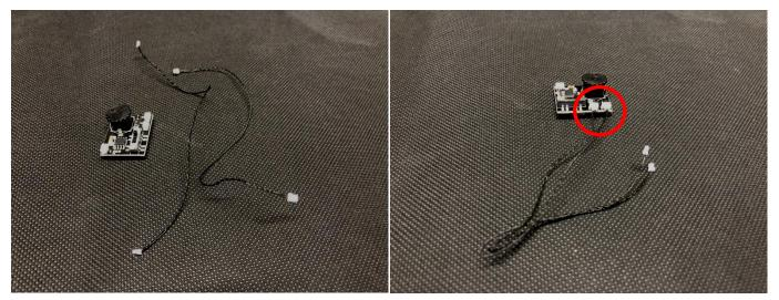
7) stick the Multi Effects Board to the bottom of the boat by sing the adhesive squares. Connect the blue strip light from the previous step to it
