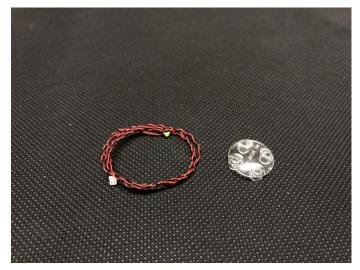
18) remove the top of the beacon, with lighting part facing up, secure the light to the top part, reconnect the top. Thread the cable through the hole in the middle of the brown
