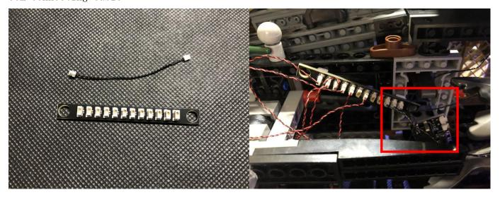
Take a USB cable, connect it to the expansion board, turn the power on to verify the current
