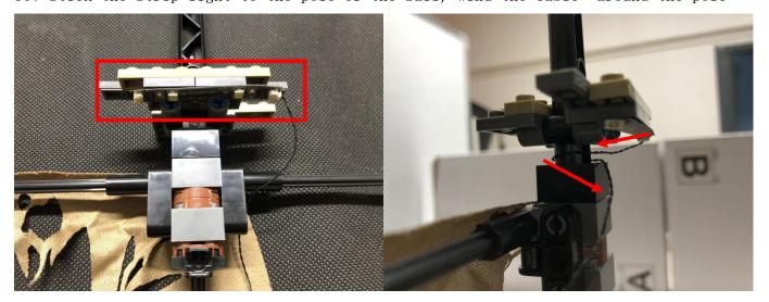
31) thread the cable through the hole on the pole, pull the cable to the cabin, connect it to the expansion board underneath
