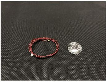
10) remove the top of the beacon, with lighting part facing up, connect the light to the top part, reconnect the top back to the beacon
