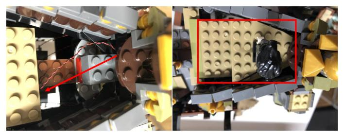
21) continue to thread the cable through the hole on the pieces underneath the boat, connect the connector to the expansion board
