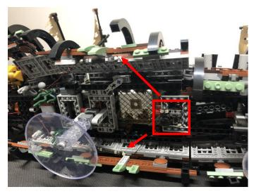
8) take a 5cm connecting cable, a 12-port expansion board, stick the expansion board to the bottom of the boat, connect the expansion board and the Multi Effects Board by using the 5cm connecting cable
