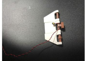
Wrap the wire around the mast and install it back on board.
