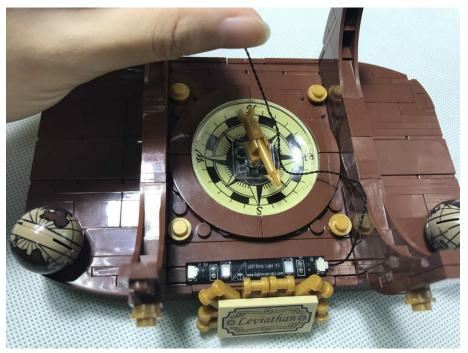
Remove the block from the side of the compass, press the cable against the stud gap, and restore the blocks.
