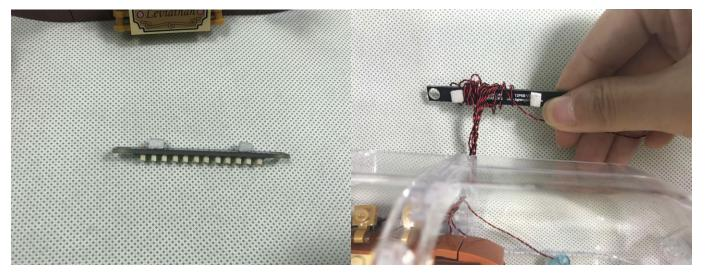
Stick the board in place, connect the power, and place the power on the side of the base.
