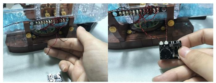
Connect the 5 cm cable to the output (only one side of the interface).
