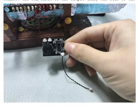
Connect the other end of the 5cm cable to the 12-port expansion board and use an adhesive square to attach the Multi-EGects Board to the base. Turn on the power, we can see that the blue dot light are flickering like a tide, you can adjust the flashing mode by shifting the gear, turn the twist to adjust the flashing speed.
