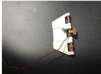
Wrap the wire around the mast and install it back on board.
