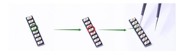
When installing dot lights, make sure they are correctly placed (Yellow LED package is exposed). You can put they either on the top of the studs or between studs.
