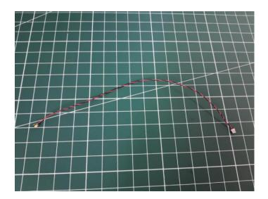
Save some length, connect it to the expansion board, and tuck excess cable around the expansion board.
