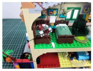
Stick the light to the roof of the left room, and stick the expansion board to the following place.
