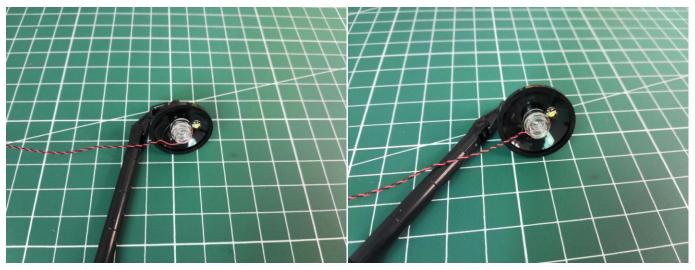
Thread the cable through the following hole.
