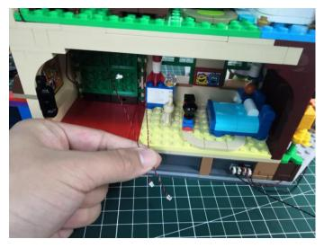
Take a 5cm connecting cable, a Flicker Effects Board, connect the cable to the IN port on the Flicker Effects Board.
