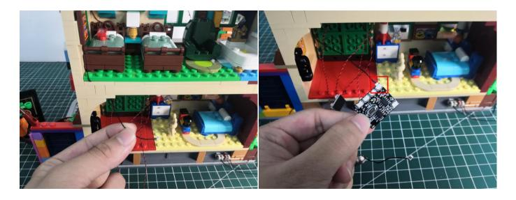
Connect the cable from the expansion board at the first floor to the  $\ensuremath{\mathsf{B}}$  port.
