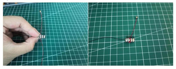
Connect the following 2 cables to the expansion board, and tuck excess cables around the expansion board.
