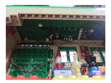
This completes installation of this LED Lighting Kit. ENJOY! (A port: lights from the second floor; B port: lights from the first floor; C port: lights from the side house; D port: street light.)
