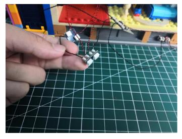
Stick 4 adhesive squares to the back of the Remote Control Switch Board.
