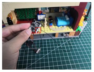
Connect the cable from the street lamp to the D port.
