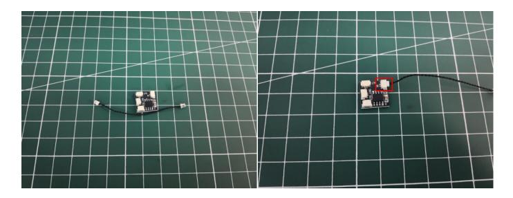
Connect the 2 cables from the wall lamps to the OUT ports on the Flicker Effects Board.
