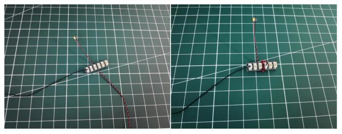
Turn to the left room, connect all the cables to the expansion board, and tuck excess cables around the expansion board.
