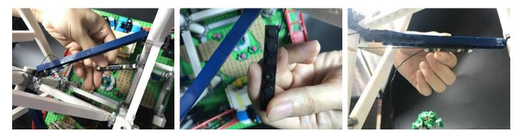
18) Thread the connector end of the 15cm cable through the hole on the blue piece, round it one time on the white pole then, downward through a hole of another blue piece
