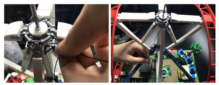
15) Pull the cable down and through the hole inside the blue piece, then, wind it around the blue piece twice
