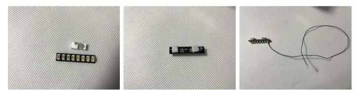
81) Connect the cables of the lights to the expansion board, stick the expansion board at the back of the house, reconnect the house section.
