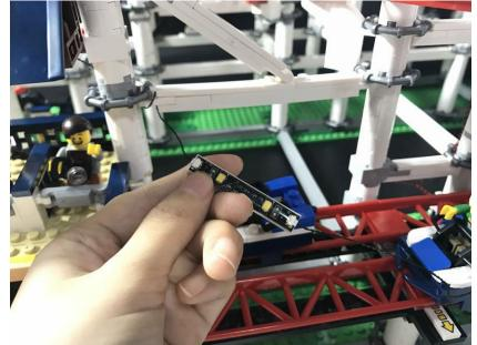
30) Wind the cable as per below, and stick the strip under the white beam
