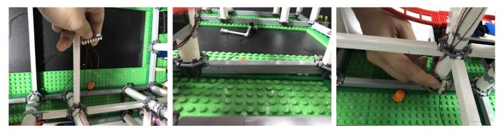
70) Thread the connector side of the 30cm cable through the hole of the gray piece
