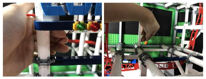
68) Take a 8-port expansion board, stick the adhesive tapes on its back, connect a 30cm cable to it
