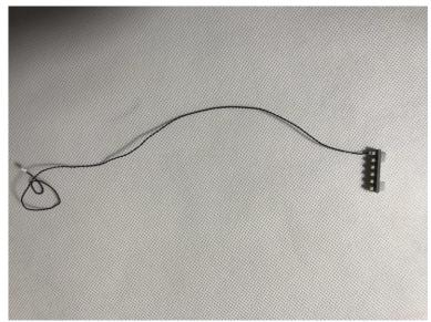
83) Pull the cable from expansion board at the back of the house to the right side of the console, connect it to the 6-port expansion board, then, stick the expansion board at the bottom of the pole.
