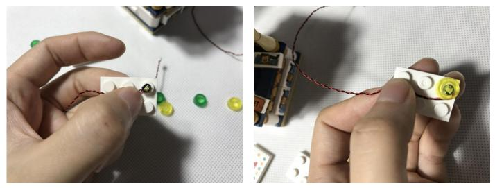
76) Repeat the previous steps to install all the 6 dot lights. Ensure you press the cables in between the studs
