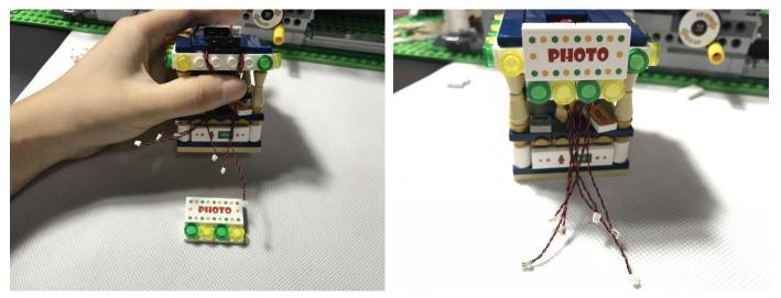
80) Take a 8-port expansion board and 2 pieces of adhesive tapes, stick the tape at the back of the expansion board, connect a 30cm cable to it
