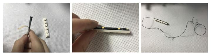
29) Connect the cable(from step27) to the other end of the strip
