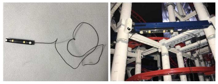
53) Wind the 50cm cable around the pole , pull it up, wind it around the gray gaps at the third and the forth level
