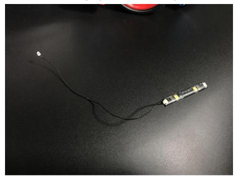
Uncover the tape at the back of the strip, stick it to the top of the car, pull the cable out from the right
