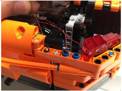
Rest the LED end of the **White 15cm Dot Light** on top of the black technic pin in the orange technic liftarm piece. Make sure the yellow LED element facing upwards. Hold this **White 15cm Dot Light** in place and….
