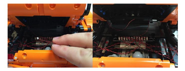
Feed the **AA Battery Pack** wire underneath the boot and plug it in to the last available port on the **12 Port Expansion Board**.
