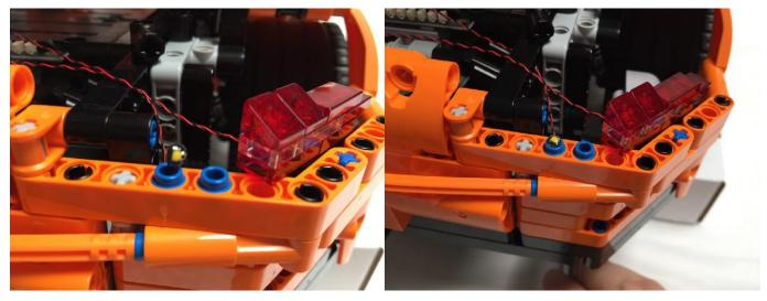
Grab the top of the LED on the **White 15cm Dot Light** and carefully bend it so that it faces upwards. You want it to sit flat on top of the blue technic 1/2 pin.
