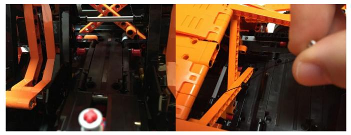
Run the **30cm Connecting Cable** in between the drivers seat and centre console. Pull it out the back "window" above where the two orange technic liftarms cross over.
