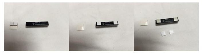
Turn the **8 Port Expansion Board** face down, peel the two **Adhesive Squares** and stick them on to the **8 Port Expansion Board**.
