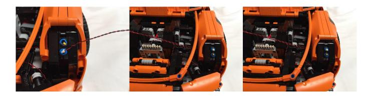
Grab another **White 15cm Dot Light** and feed it through the bottom blue technic 1/2 pin. Carefully bend the end of the LED element so that it will sit flat on top of the blue technic 1/2 pin when it is pulled through.
