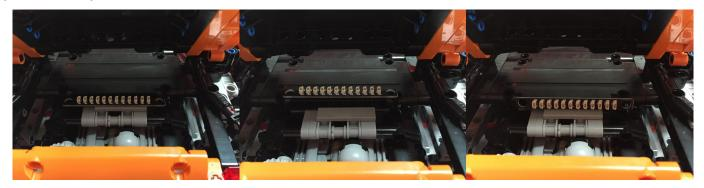
There are a few options for mounting the **12 Port Expansion Board**. I am going to mount mine on top of the 1 x 4 tile. If you have applied a sticker to this piece, you may want to mount the expansion board in one of the other positions shown in the photos above.
