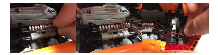
Repeat the process for all remaining wires. When you have finished this side, there should be five wires plugged into the **12 Port Expansion Board**.
