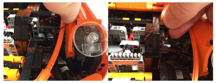
Run the plug ends of the **White 15cm Dot Lights** we just installed up and through the double size holes on the black technic liftarms near the **8 Port Expansion Board**.
