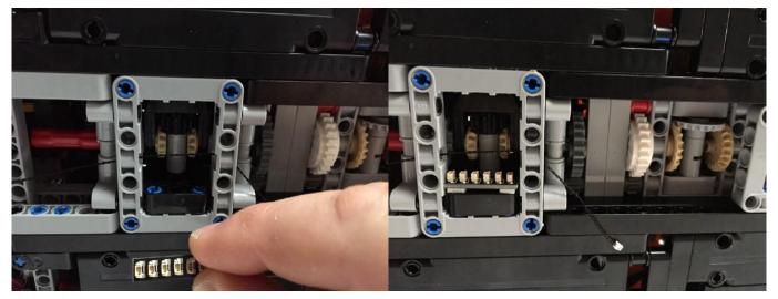
Stick the **6 Port Expansion Board** on to the side of the 1 x 3 black technic liftarm, which is inside the rectangle technic piece that is roughly in the centre of the car.
