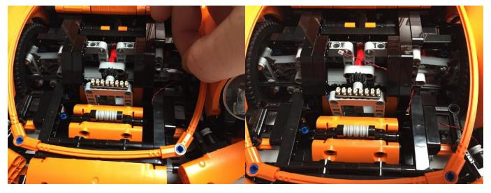
Now run the plug end of the **White 15cm Dot Light** up and through the double size holes on the black technic liftarms near the **8 Port Expansion Board**.
