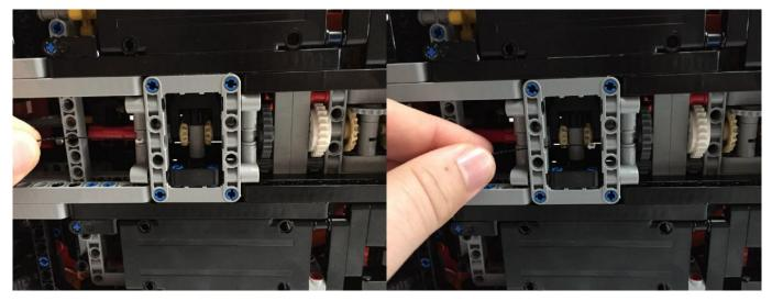
Pull the **30cm Extension Cable** through and feed it through the available centre holes in the rectangle technic piece that is roughly in the centre of the car.
