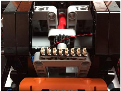
Plug the **White 15cm Dot Light** into and available port on the **8 Port Expansion Board**.
