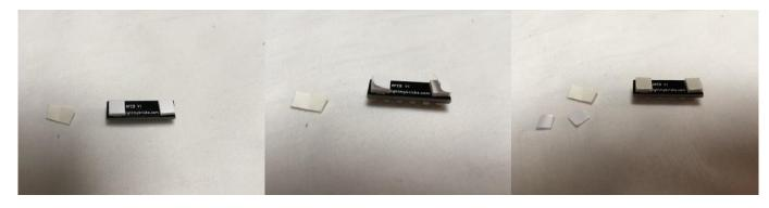
Peel the **Adhesive Squares** off the base and stick them to the back of the 6 **Port Expansion Board**. Remove the top bits of paper to expose the other sticky side of the **Adhesive Squares**.
