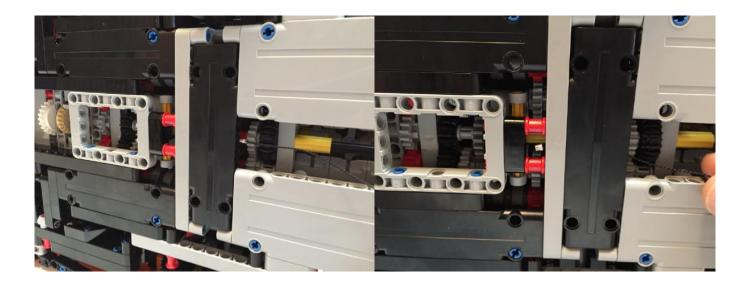
Now run the **50cm Connecting Cable** towards the front of the car. Feed the cable through the side holes of the black technic panel plate.
