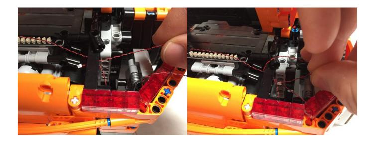
You will have four **White 15cm Dot Lights** that need to be plugged into the **12 Port Expansion Board**. Two are likely to be easily accessible and the other two have run down under the car. Gather the wires one at a time and feed them through the black technic liftarm piece. Wrap them around the black technic liftarm piece as appropriate to consume any slack in the wires.
