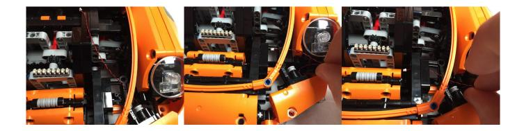
Grab the plug end of the **Cool White 15cm Dot Light** and feed it through available holes in the side of the black technic lift arms as seen in the picture above.
