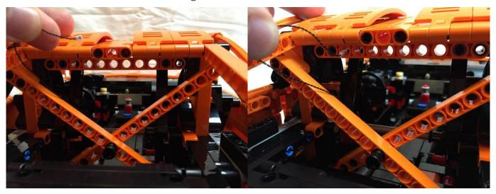
Feed the **30cm Connecting Cable** through an available hole in the orange technic liftarm that runs underneath the roof line.
