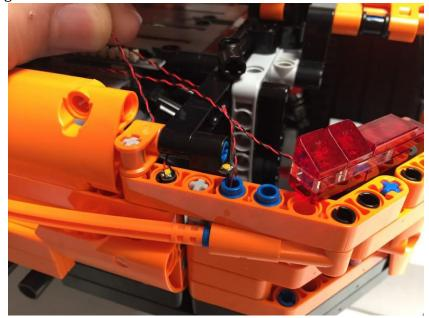
Rest the LED end of the **White 15cm Dot Light** on top of the black technic pin in the orange technic liftarm piece. Make sure the yellow LED element facing upwards.
