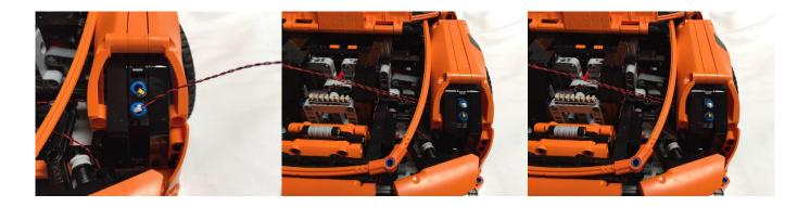
Grab another **Cool White 15cm Dot Light** and feed it through the bottom blue technic 1/2 pin. Carefully bend the end of the LED element so that it will sit flat on top of the blue technic 1/2 pin when it is pulled through.
