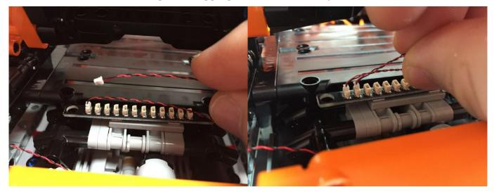
Plug the wires into available ports on the **12 Port Expansion Board**.
