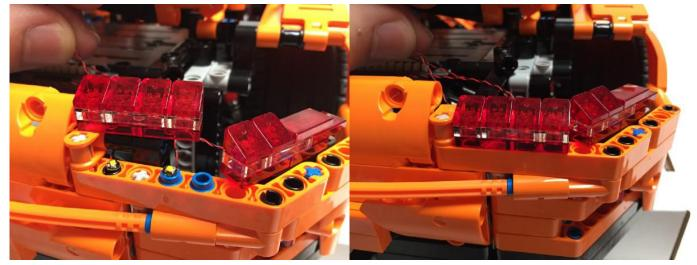
Replace the transparent brake light pieces. Each **White 15cm Dot Light** LED will sit comfortably inside the cavity of the Lego plate being fixed on top of it. No extra resistance should be encountered when refitting the brake light pieces.
