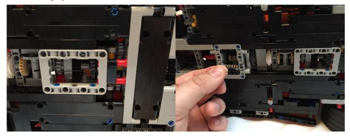
Pull the wire through and it should reach somewhere near the 6 Port Expansion Board.
