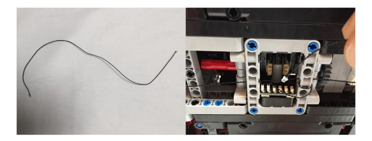
Grab the other **30cm Connecting Cable** and connect it to an available port on the **6 Port Expansion Board**.
