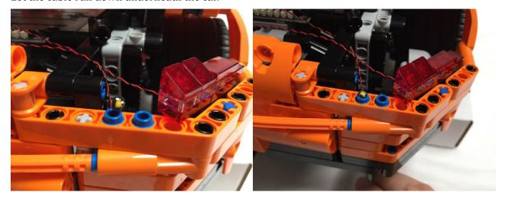
Grab the top of the LED on the **White 15cm Dot Light** and carefully bend it so that it faces upwards. You want it to sit flat on top of the blue technic 1/2 pin.
