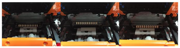
There are a few options for mounting the 12 Port Expansion Board. I am going to mount mine on top of the  $1 \times 4$  tile. If you have applied a sticker to this piece, you may want to mount the expansion board in one of the other positions shown in the photos above.
