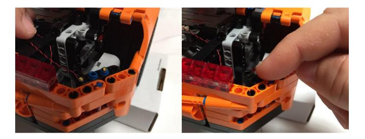
The blue technic 1/2 pins sit inside a black L-Shaped technic lift arm. There is a black technic pin in the corner of the black L-Shaped technic lift arm. Grab a **White 15cm Dot Light** and rest it on top of the black technic pin with the yellow LED element facing upwards.
