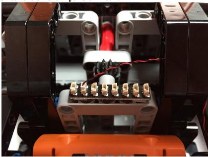
Plug the Cool White 15cm Dot Light into and available port on the 8 Port Expansion Board.
