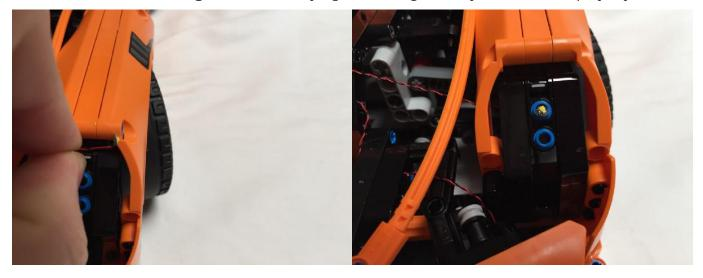
Carefully bend the end of the LED element so that it will sit flat on top of the blue technic 1/2 pin when it is pulled through.
