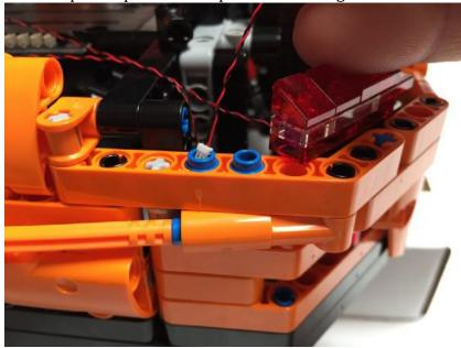
Again, two blue technic 1/2 pins will now be exposed. Grab a **White 15cm Dot Light** and feed the white plug end through the blue technic 1/2 pin closest to the centre of the car. Let the cable run down underneath the car.
