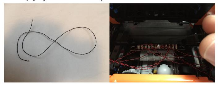
Open the boot, grab the **50cm Extension Cable** and plug it into an available port on the **12 Port Expansion Board**.
