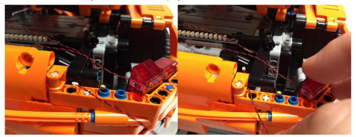
Grab a **White 15cm Dot Light** and feed the white plug end through the available gap between the orange technic liftarm (that holds the blue 1/2 technic pins) and the black technic liftarm that runs back towards the engine.
