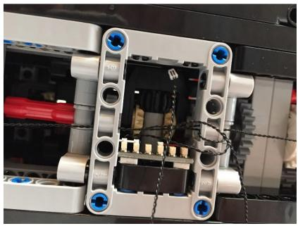
Feed the **30cm Connecting Cable** up through the available hole in the side of the technic rectangle piece. The cable runs vertically up and away from the **6 Port Expansion Board**.
