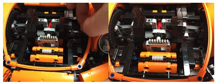
Now run the plug end of the **Cool White 15cm Dot Light** up and through the double size holes on the black technic liftarms near the **8 Port Expansion Board**.
