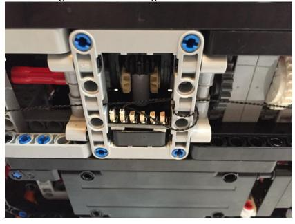
Plug the **50cm Connecting Cable** into the **6 Port Expansion Board**.
