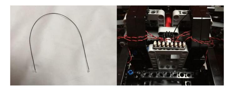
Grab the 30cm Extension Cable and plug it in to an available port on the 8 Port Expansion Board.
