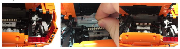
Plug the **White 15cm Dot Light** into an available port on the **12 Port Expansion Board**. I have chosen the furthest port on the left to minimise the amount of slack in the wire.
