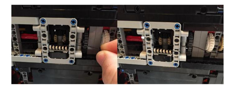
Feed the **50cm Connecting Cable** through the centre hole in the side of the technic rectangle piece that has the **6 Port Expansion Board** in it.
