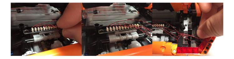
Repeat the process for all remaining wires. When you have finished this side, there should be five wires plugged into the 12 Port Expansion Board.
