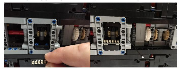
Stick the **6 Port Expansion Board** on to the side of the  $1 \times 3$  black technic liftarm, which is inside the rectangle technic piece that is roughly in the centre of the car.
