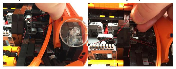
Run the plug ends of the **Cool White 15cm Dot Lights** we just installed up and through the double size holes on the black technic liftarms near the **8 Port Expansion Board**.
