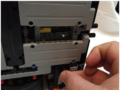
Grab the end of the **50cm Connecting Cable** and feed it through the holes in the side of the technic panel plate. Run the cable from the outside of the technic panel plate towards the centre of the car.
