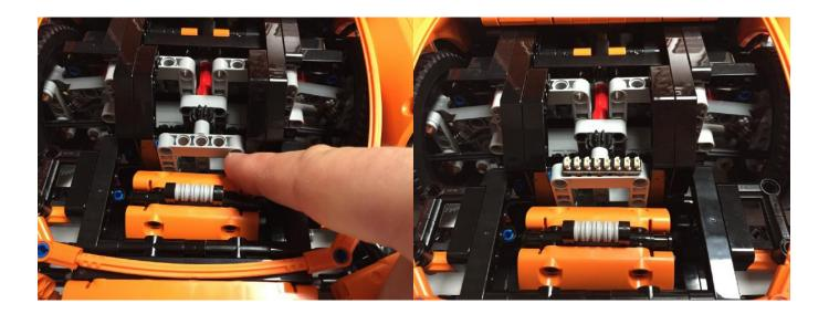
Mount the **8 Port Expansion Board** on top of the rectangle technic piece as shown in the picture above.
