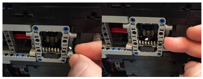
Depending how much excess cable you have, wrap the **50cm Connecting Cable** around the technic rectangle piece and feed it through the centre hole again.
