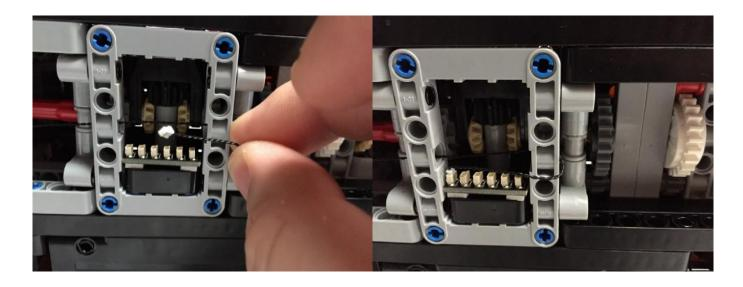
Grab the **30cm Extension Cable** and plug it into the best port on the **6 Port Expansion Board** that leaves the least amount of slack in the cable.
