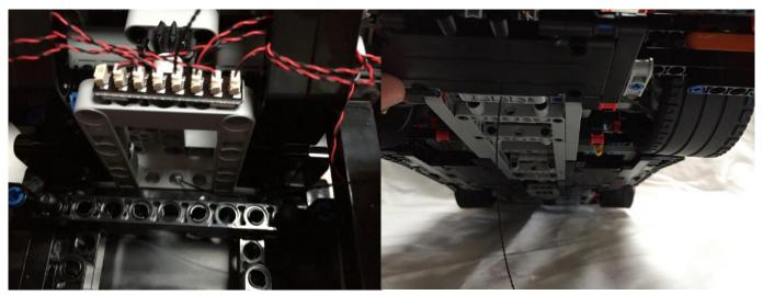
Feed the other end of the **30cm Extention Cable** through the centre hole in the bottom of the same rectangle technic piece that the **8 Port Expansion Board** is attached to.
