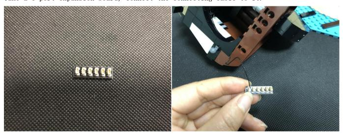
Stick the expansion board to the bottom of the ship with adhesive squares.
