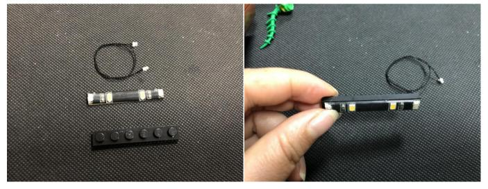
Connect the connecting cable to the strip light, connect the following connecting cable to the spare end of the strip light.
