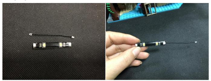
Connect the connecting cable from the strip light to the expansion board.
