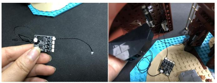
Take the USB cable, connect it to the power port on the Remote Control Switch Board as per below.
