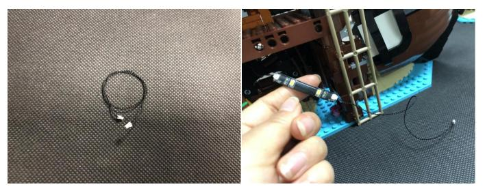
Stick the strip light to the roof of the first floor, thread the 15cm connecting cable through the following space to the ladder.
