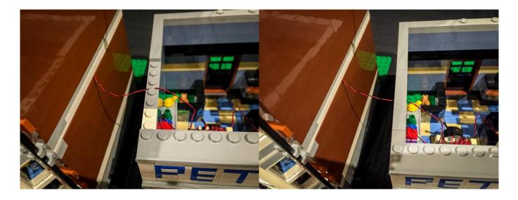
20.) Connect the 15cm cable we connected to striplight#1 from the red building into a spare port of the expansion board then take another 15cm cable and connect it into the final port on the expansion board.
