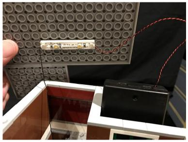
Secure the battery pack and cable in place by connecting them underneath the grey Lego tiles.
