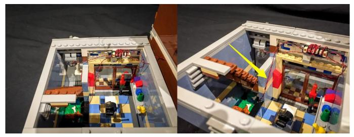
21.) Take the 2nd level and place it on top of the ground floor. Tip it on its back and connect/stick a strip light (**Striplight#5**) to the bottom of it in the following position. Connect the other end of the 15cm cable we connected earlier to the expansion board into the left port of the strip light.
