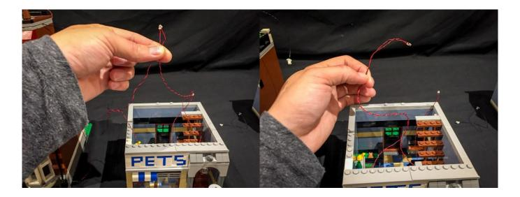
Take the **6-port expansion board** from this kit and connect the 2 cables we twisted together into the the spare ports of the expansion board. Wind the 2 cables around the expansion board to free up the excess cable as per below.
