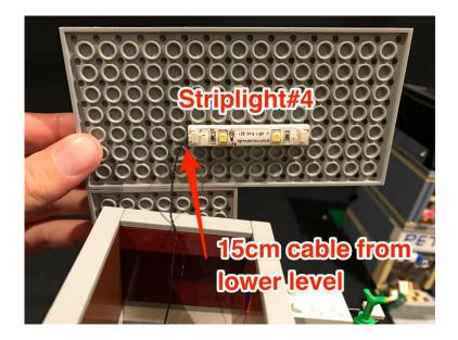
12.) Take the **AA Battery pack** and insert 3 AA batteries into it. Place the battery pack on the balcony and then insert the attached cable into the right port of striplight#4.
