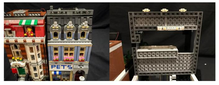
Take another 15cm cable and connect this to the left port of striplight#6. Thread this up and pull it up from the top of the floor and set aside ensuring it does not drop back down below. Locate the 15cm cable we pulled up from the door on the level below and connect this to the right port of striplight#6. Reconnect the entire 3rd floor back in place.
