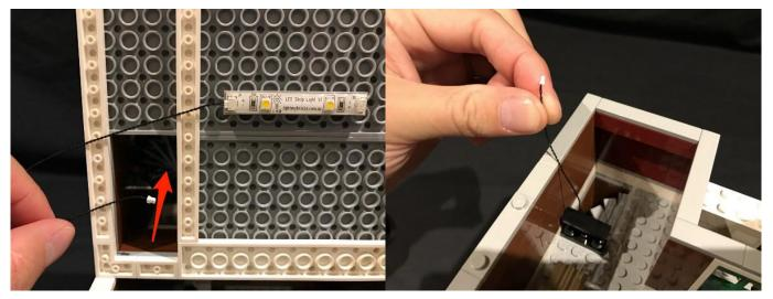
8.) Take the 3rd level and then turn it on its back so that we can see underneath. Take another 2 strip lights and connect them together using a **5cm connecting cable**, then connect/stick them in the following positions. These will be identified as **striplight#2** and **striplight#3**.
