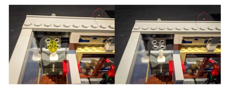
16.) Take a Dot Light and place it in the middle of the 4 grey studs ensuring the LED component part is facing the correct way up. Secure this Dot Light in place by reconnecting the transparent yellow Lego light piece directly over the top. Ensure that the cable is facing the same way as per below. The Dot Light should sit comfortably in the middle of the light piece. Once this is done, reconnect the transparent globe piece over the top.
