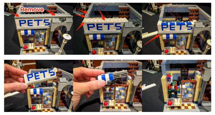
Take the below pieces and then install another Dot Light to the bottom of the blue and white roof. Secure the Dot Light in place by reconnecting the brown window underneath ensuring that the Dot Light cable is facing the inside of the building and laying in between the brown studs. The LED component should be visible if you look from underneath.
