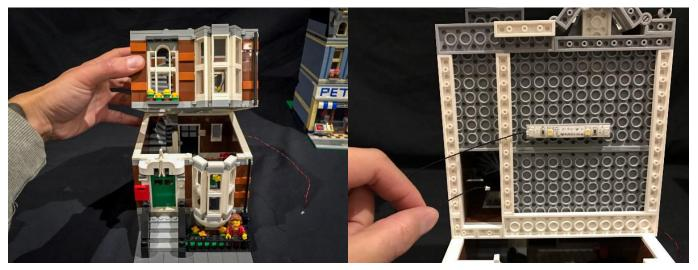
6.) Take another 15cm cable and connect it to the right port of the strip light. Secure this cable by reconnecting the white lego plate over it.
