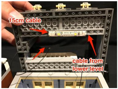
24.) Pull the 15cm cable up from the below 2nd floor and connect it to the final strip light (striplight#7). Take the roof of the building and connect/stick the strip light in the below position.
