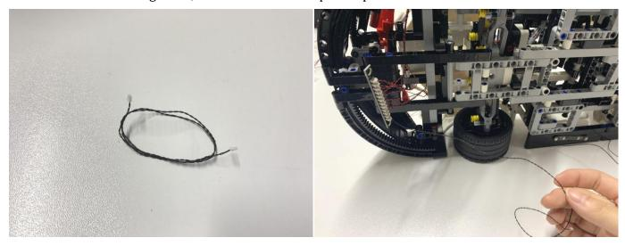
Stick tapes at both sides of the expansion board, tuck excess cables around the board, then, stick the expansion board to the inside of the car
