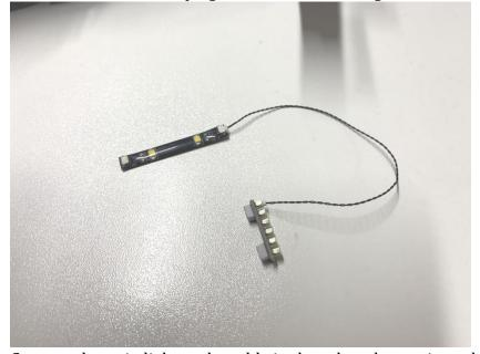
Connect the strip light to the cable in the cab and paste it on the roof
