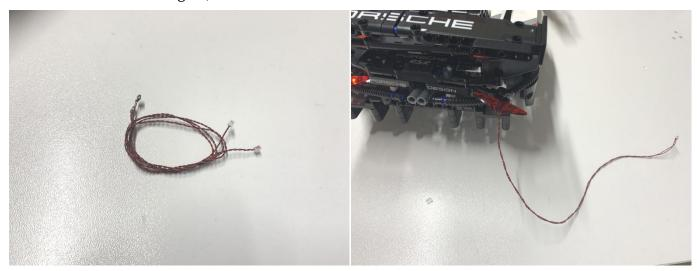
Connect them to the 6-port expansion board, turn the battery pack on, then check if the lights are working OK .Place the cable underneath the battery pack
