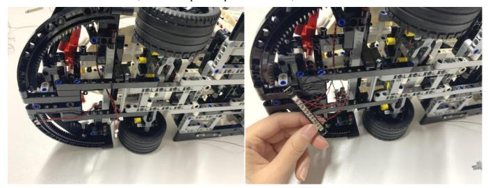
Take a 30cm connecting cable, connect it to the 12-port expansion board
