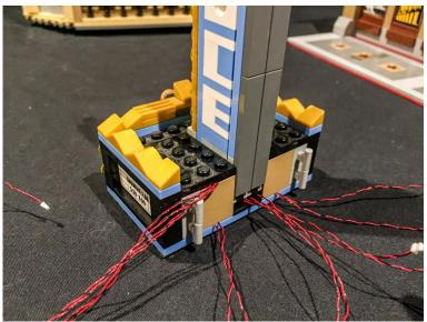
48.) Take another 12-port expansion board (**Expansion board#3**) and connect a 5cm cable to one side and a 15cm cable to the other side.
