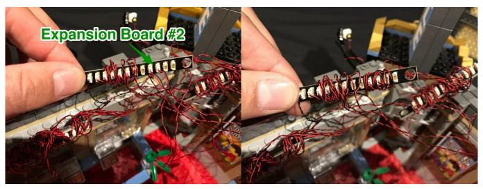
53.) Connect Expansion board#2 and Expansion board#3 to each other by using the 5cm connecting cable.
