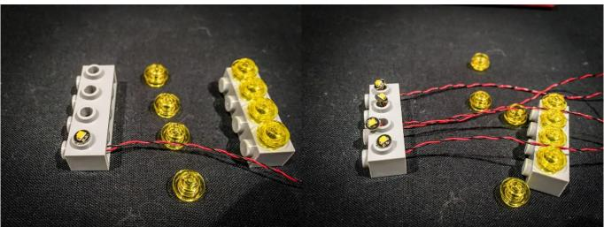
Ensure LED component is facing the correct way up
