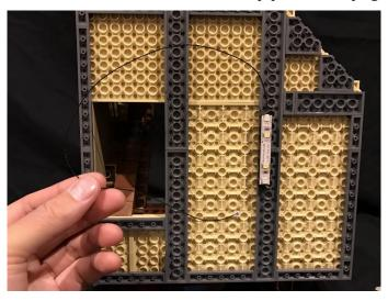
Connect this to the rest of the circuit by connecting the 15cm cable from Expansion board#3 to the bottom port of striplight#1.
