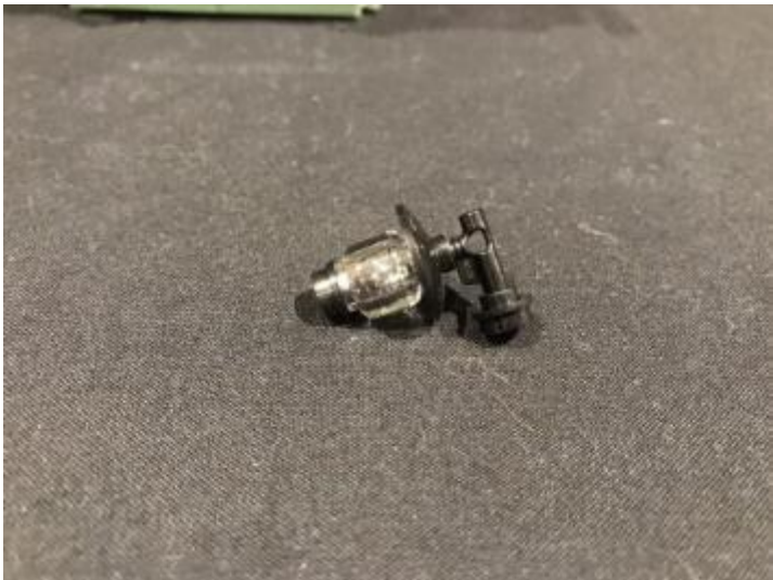
Remove the lamp at the bottom of the section, disassemble the black stud
