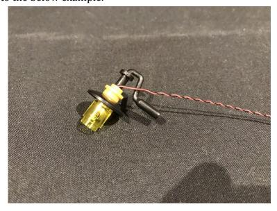
Lastly, reconnect the remaining piece which sits underneath the lamp before reconnecting back to the front mast.
