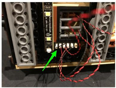
29.) Pull all the excess cables down and twist them together before tucking them inside underneath the grey 2x8 plate.
