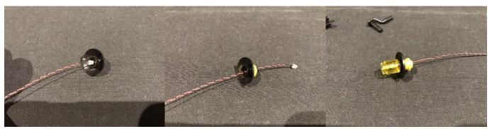
Reconnect the black hook piece by carefully pushing down through the top of the lamp shade piece. *NOTE: You will notice that this particular piece will not push all the way down. Do not force push it all the way.*
