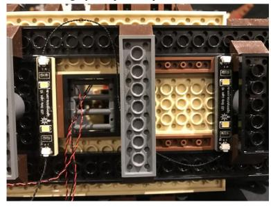
28.) Use the provided **double sided adhesive squares** to mount the expansion board to the following position.
