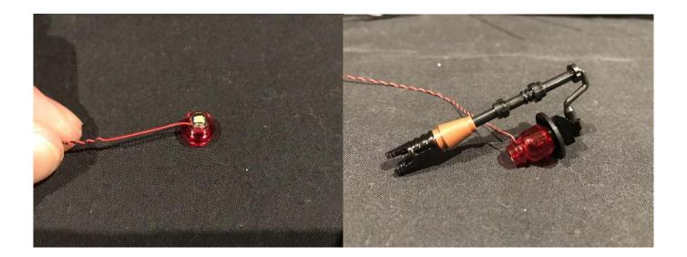
Wind the cable around the pole and then reconnect this section to the side of the boat.
