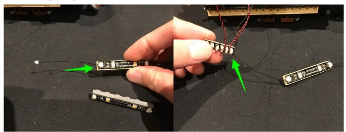
27.) Connect both strip lights underneath the upper level section in the below positions. Ensure the strip light with the spare port is closest to the back of the ship.
