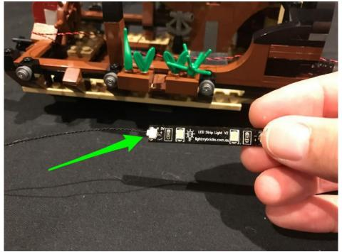
Using the adhesive backing, stick the strip light underneath the roof of the upper deck in the following position. The Strip Light should be placed in the middle between the two front roof flaps.
