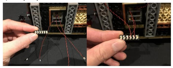
26.) Take **2x White Strip Lights** and then stick them (using their adhesive backing) onto the base of the **2x provided LEGO 1x6 Plates**.
