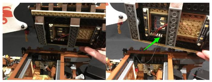
31.) Before reconnecting the upper level, take the **AA Battery Pack** and place it behind. Connect the battery pack cable into the strip light towards the back.
