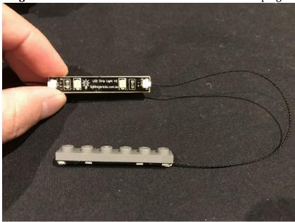
Take a **5cm Connecting Cable** and connect it to one of the strip light ports and then connect the other end into the 6-port expansion board.
