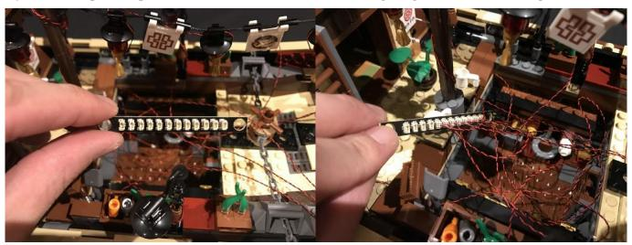
Take this time to test all lights are working ok by taking the the **AA Battery Pack** and inserting 3x AA batteries into it. Take the battery pack cable and connect it to one of the available ports on the expansion board. Turn the switch ON and verify that all lights are working OK.
