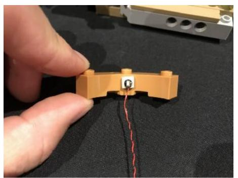
Reconnect the brown LEGO brick and then secure the cable in place by disconnecting the other brown LEGO brick opposite, laying the cable and then reconnecting back over the cable. Ensure the cable underneath is laid in between studs.
