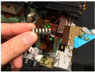
17.) Take a **White Strip Light** and stick it to the base of another LEGO 1x6 plate. Connect a **5cm connecting cable** to the left port of the strip light and then connect the other side of the cable to the expansion board.
