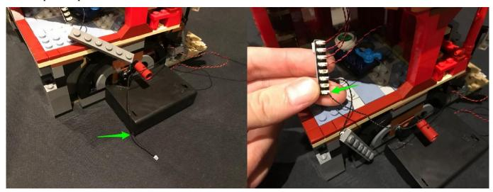
Using **2x Adhesive Squares**, mount the 8-port expansion board as well as the the White Strip Light on to the ceiling of the bottom floor as per below:
