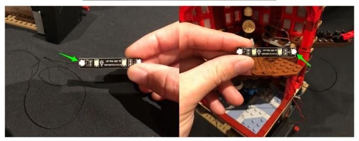
Mount the Strip Light to the ceiling of the middle level at the following position. Ensure the connected 30cm cable is facing the inside of the temple.
