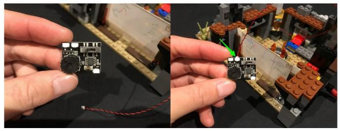
To configure the effect, we are going to require power so take the **AA Battery pack** and insert 3x AA batteries to it. Connect the Battery Pack cable into the input port (side with 1 port) and turn on. Set the switch all to the far left for the "flicker" effect (to give the water fountain a realistic flickering water look) and then turn the wheel to adjust the speed of the effect.
