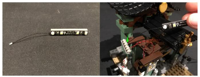
Thread the strip light through the space inside of the roof and then mount it underneath to the following position.
