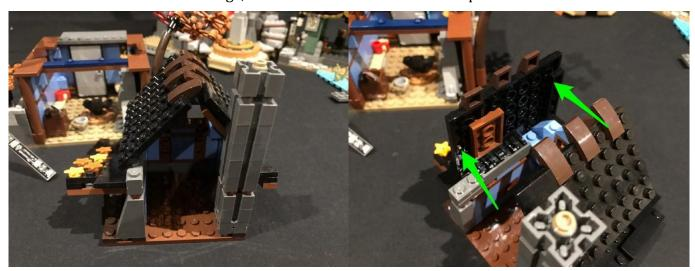
With the cable facing behind, mount the strip light to the following position on the left side of the roof and then close the roof.
