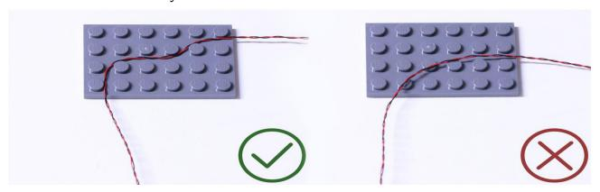
Insert the connectors to the ports.
