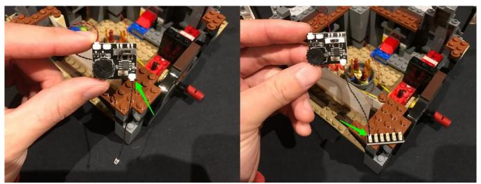
Take **2x 50cm Connecting Cables** and a **15cm Connecting Cable** and connect it to available ports on the expansion board.
