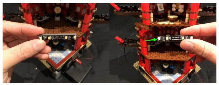
Eliminate excess cable by winding the cable around the Strip Light 4 – 5 times before mounting it to the ceiling of the top floor in the below position.
