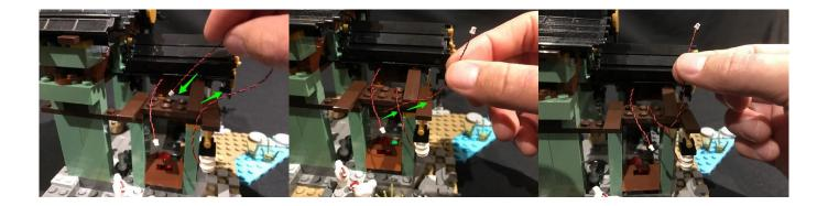
Take a **6-port Expansion Board** and connect both Dot Light cables to available ports.
