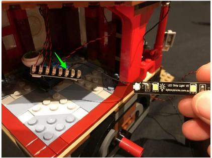
Take the other end of the 15cm cable (from the right side of the base) and connect this to another port on the 8-port expansion board.
