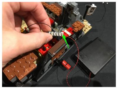
Thread one of the 50cm cables out the left side through the spacing in the corner of the building. Pull the cable all the way out from the outside.
