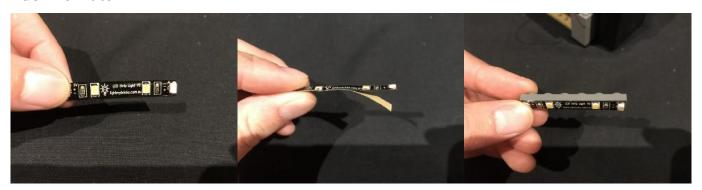
Connect a **5cm Connecting Cable** to the left port and a **15cm Connecting Cable** to the right port.
