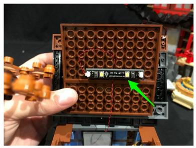
Take the 15cm connecting cable from the second floor and connect this to the right port on the strip light underneath.
