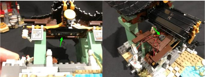
Mount the expansion board to the inside of the roof using 2x adhesive squares.
