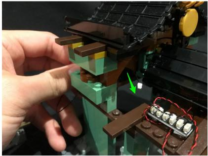
Pull the cable through and then connect it to a spare port on the 6-port expansion board.
