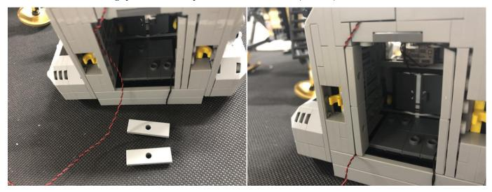
Connect the cable to the expansion board
