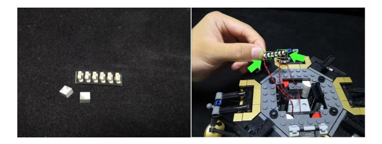
23. Take a 5cm connecting cable, connect it to the 6-port expansion board.
