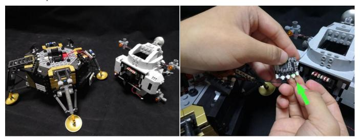
61. Connect the 15cm head light cable from the ascending part to the '4' port on the Remote Control Switch Board.
