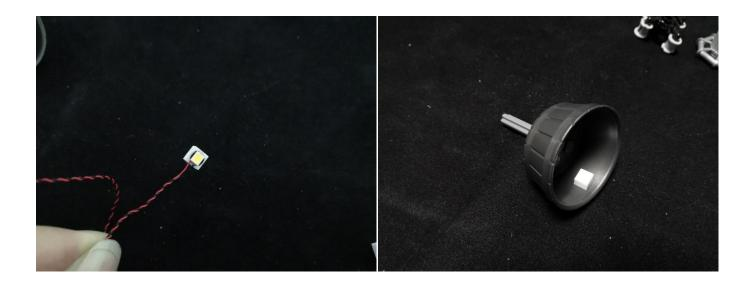
8. Stick the light to the following place, secure the cable with the other adhesive square.
