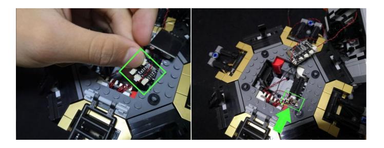
66. Stick the Remote Control Switch Board to the following place with an adhesive square.
