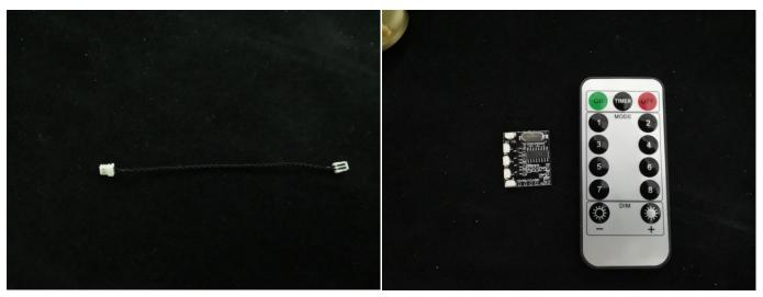
15. Connect the 5cm connecting cable to the input port on the Flicker Effects Board, connect the other end to the '1' port on the Remote Control Switch Board.
