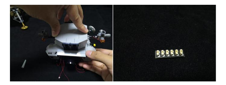
56. Connect the following cables marked in green (4 cables of the warm white dot lights) to the 6-port expansion board, (you can tuck excess cables around the expansion board).
