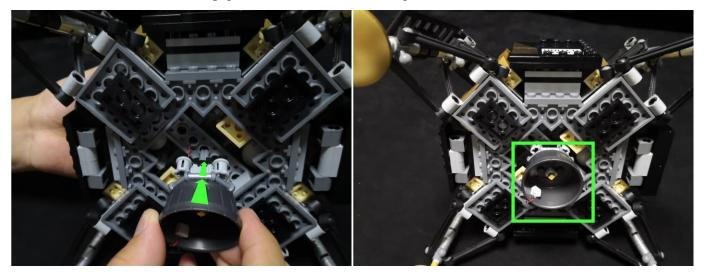
13. Turn the descending part back, connect the cable of the light to the output port on the Flicker Effects Board.
