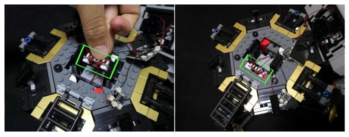
65. Tuck excess cable on the Flicker Effects Board as per below, stick it to the following place with an adhesive square. s
