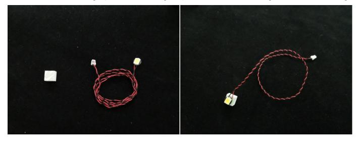
31. Stick the head light to the following place, follow the arrows to place the cable as per below.
