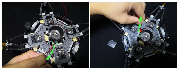
21. Turn this part over, pull the cables out (in case of breaking the cables, do not pull them too hard).
