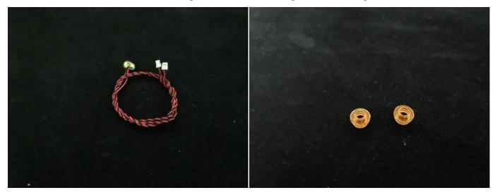
34. Thread the cable of the light though the trans orange 1x1 piece (thread it in right direction, and make sure the lighting part is facing the right direction).
