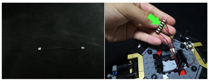
24. Connect the other end of the 5cm connecting cable to the port '2' on the Remote Control Switch Board.
