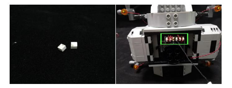
60. Take the descending part, connect the 5cm connecting cable from the ascending part to the '3' port on the Remote Control Switch Board.
