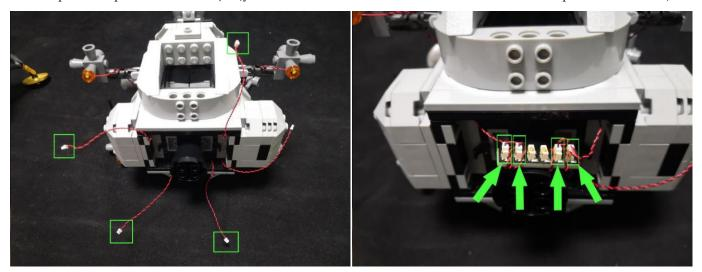
57. Take a 5cm connecting cable, connect it to the 6-port expansion board.
