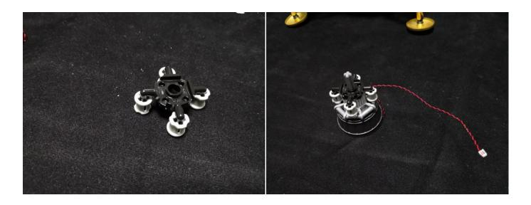
11. Turn the descending part to its side, thread the cable through the following gray piece underneath to the back.
