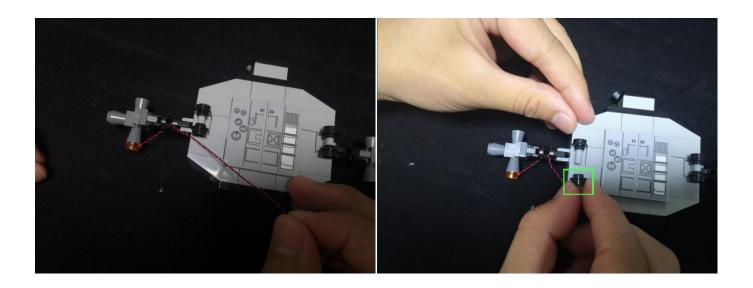
50. Press the cable underneath the following gray piece, reconnect the 1x1 black piece.
