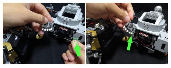
62. Take a USB cable, connect it to the input port on the Remote Control Switch Board.
