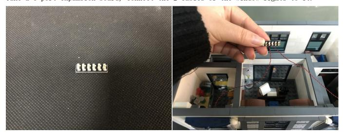
Stick the expansion board to the following place, connect the cable from the stairway to it.
