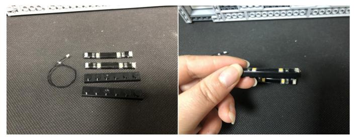
Connect the 2 strip lights together with the connecting cable, stick the 2 strip lights to the following place.
