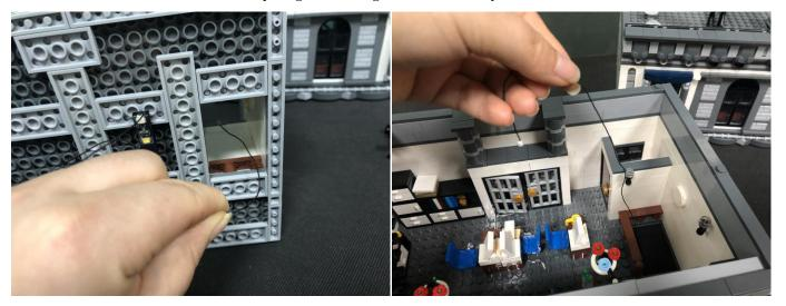
Pull the cable from the left strip light to the expansion board, reconnect the second floor.
