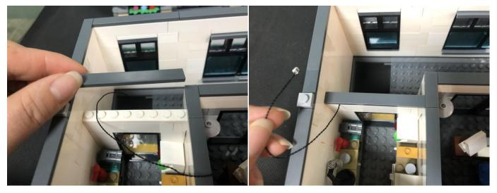
Take a 15cm connecting cable, connect it to the expansion bord at the second floor, connect the other end to the strip light at the third floor.
